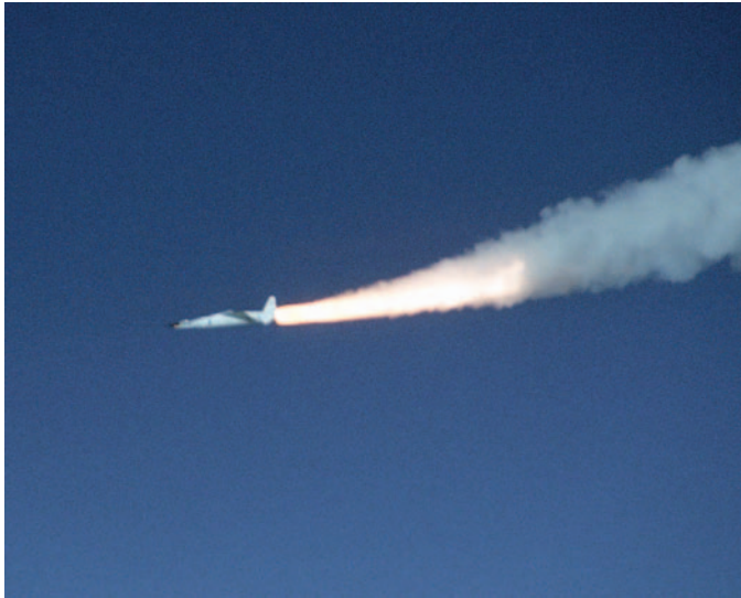
NASA's X-43A research craft set a speed record when its air-breathing engine propelled the vehicle to nearly Mach 10, or 7,000 miles per hour, in November 2004.
