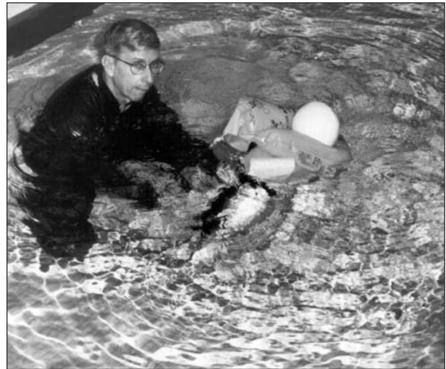
MODEL WORKER. Funkhouser working with one of CAMI’s specially constructed child dummies in assessments of the performance of various flotation devices for infants and children. In addition to performance in the water, design features, such as strap locations, may influence donning time (which would require the assistance of a parent or other adult) – another critical safety issue.
