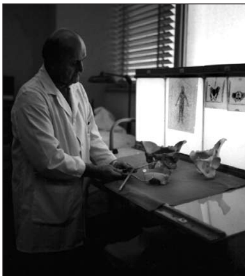
ALMOST REAL. (l) Young at work on the “golden pelvis.” Accurate pelvis representations in dummies permitted a more precise evaluation of injury in various crash scenarios.
