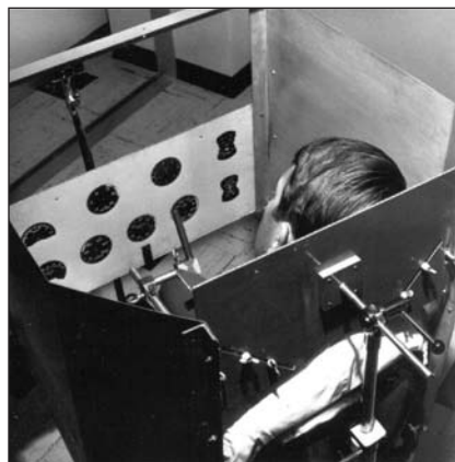
DEVELOPING AN APPLICATION. Stages in the development of CAMI's angular accelerator for vestibular research and laboratory demonstrations of spatial disorientation.
