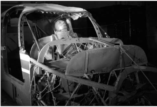
DAMAGE CONTROL. Many of Swearingen's early tests used fuselages like this one to determine where (and what) protective materials might best be located.
