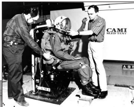
NASA NEEDS. Impact tests conducted by DeWeese (l) and Gowdy (r) in support of the NASA program occurred during the '90s. A NASA flight suit (l) was used on the dummy in one set of trials.
