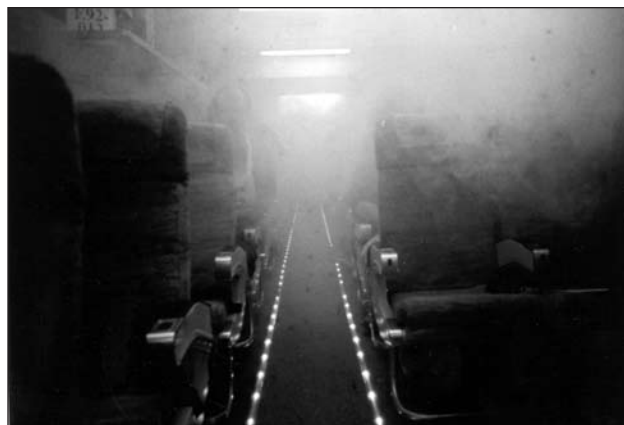
FLOOR LIGHTING WORKS. As a cabin fills with smoke, it stratifies from the ceiling down. Thus, upper level emergency lighting is obscured well before the floor-lighting "pathway" to an exit.
