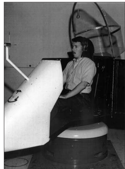
DEVELOPING AN APPLICATION. Stages in the development of CAMI's angular accelerator for vestibular research and laboratory demonstrations of spatial disorientation.
