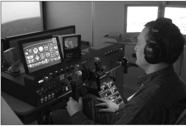
BY GAR. The BGARS “cockpit” shown here as used in the CAPSTONE project faces a large display screen with programmable flight scenarios.
