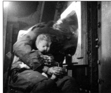
EXPLOSIVE DECOMPRESSION. An early study by Swearingen used Elmer – and a doll – to assess the effects of a rapid decompression from a blown-out window in an altitude chamber. Swearingen's recommendations related to window size, use of double panes, and an increased distance of the passenger from the window. In developing his recommendations, Swearingen exposed himself to a number of rapid decompressions.
