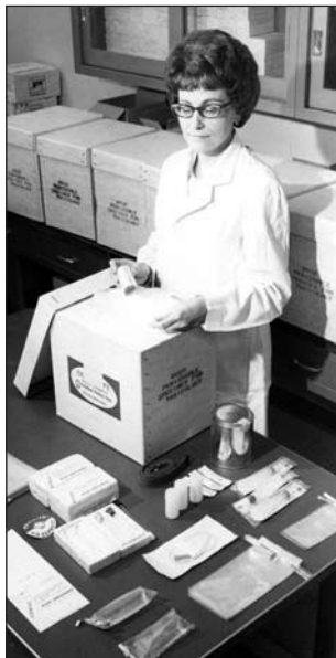
ACCIDENTS AND THE “TOX BOX”. CARI/CAMI’s famous “tox box” kits at Flight Standards District Offices contain instructions and materials to obtain samples from a fatal aircraft accident to be packed and shipped to CAMI for analyses. Precise documentation of all evidence received by CAMI is carried out in a modern accessioning laboratory.
