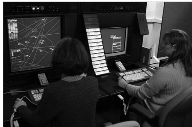
ATCARS. This innovative capability developed by Dennis Rester provides a means of testing new air traffic control equipment and procedures and their effects on workload, performance, and situation awareness.
