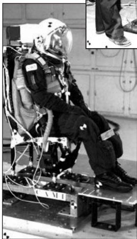
NASA NEEDS. Impact tests conducted by DeWeese (l) and Gowdy (r) in support of the NASA program occurred during the '90s. A NASA flight suit (l) was used on the dummy in one set of trials.
