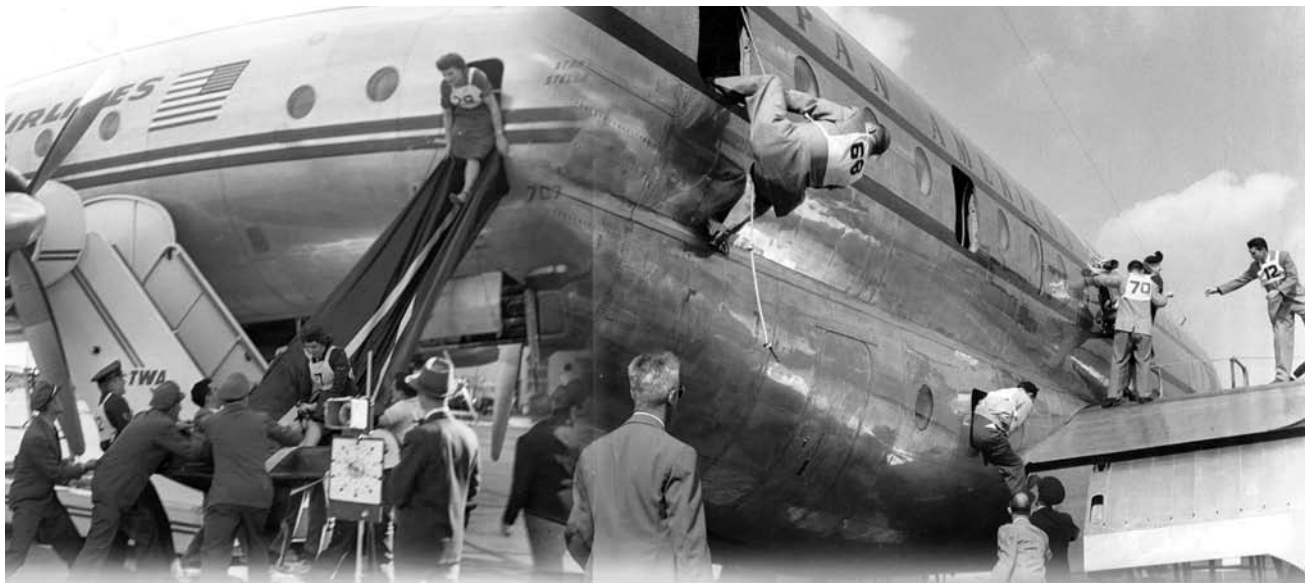
The Way It Was. Into the 1960s, prior to tricycle landing gears and the resulting higher aircraft profiles, emergency escape procedures were rudimentary. Some airlines used ropes and one carrier used a Jacob's ladder. The "telescope" pole (like a fireman's pole, but collapsible for storage) was another approach initially explored. The first escape slides were sheet-like and had to be held by those on the ground.
