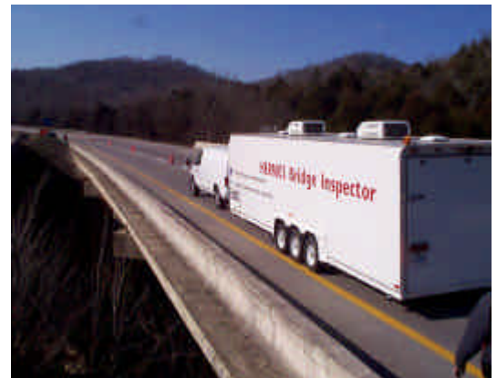
HERMES Bridge Inspector performing radar imaging of a bridge deck outside Nashville, TN.
