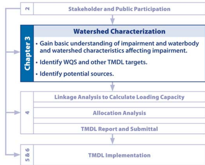
Figure 4. Illustration of the steps in the TMDL process, including the step of watershed characterization discussed in this chapter.
