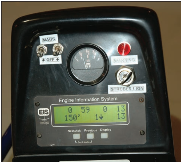
Figure 3-7. Typical engine information system.
