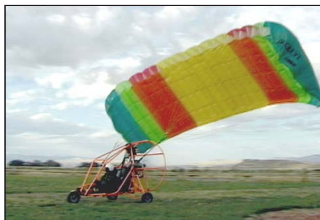
Figure 12-4. A wing lock-out.
