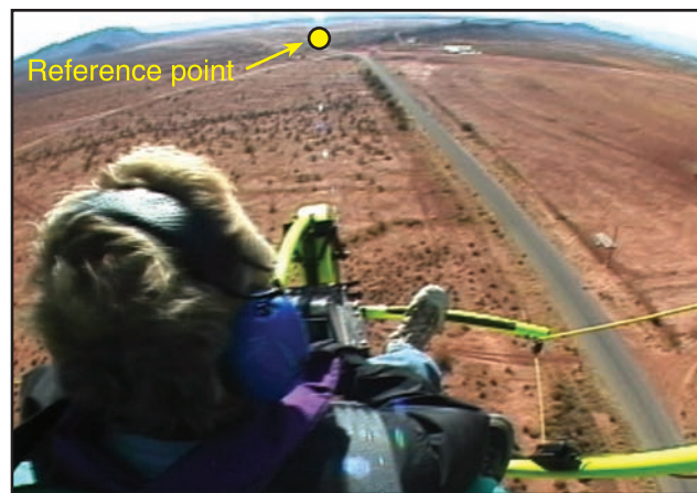
Figure 6-4. Nose reference for straight-and-level flight.
