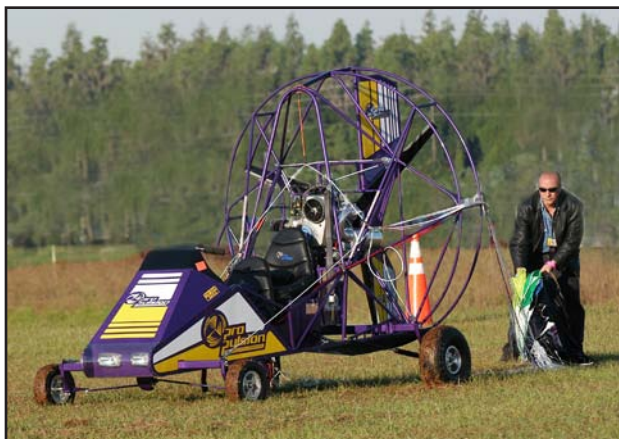
Figure 12-2. Secure the PPC wing when on the ground.
