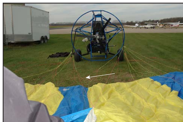
Figure 5-14. “X” in the suspension lines marks the exact center of the uninflated wing.
