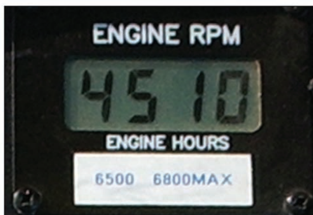
Figure 4-5. Engine RPM is indicated on the gauge.
