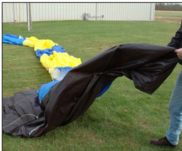
Figure 5-21. A simulated line-over.
