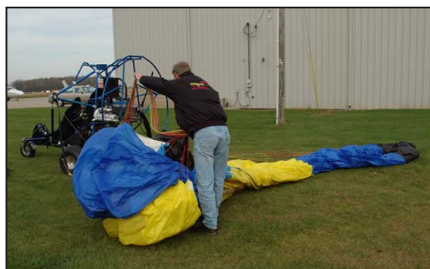
Figure 5-20. Pilot throwing the wing edge through to undo a line twist.
