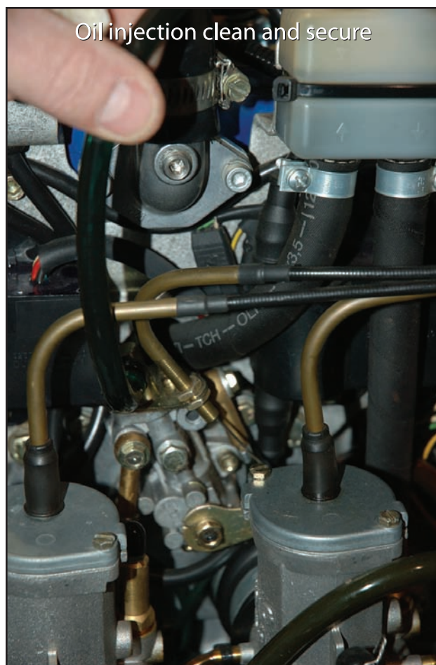
Figure 5-7. Check the ignition switches, primer and oil injections mechanism during preflight inspections.
