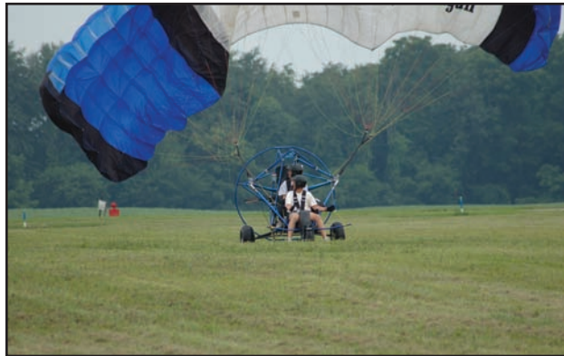
Figure 11-7. Collapsing the parachute.
