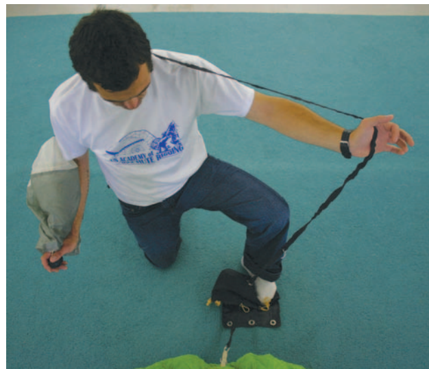
Figure 4-21. If used, cock the kill-line bridle.
