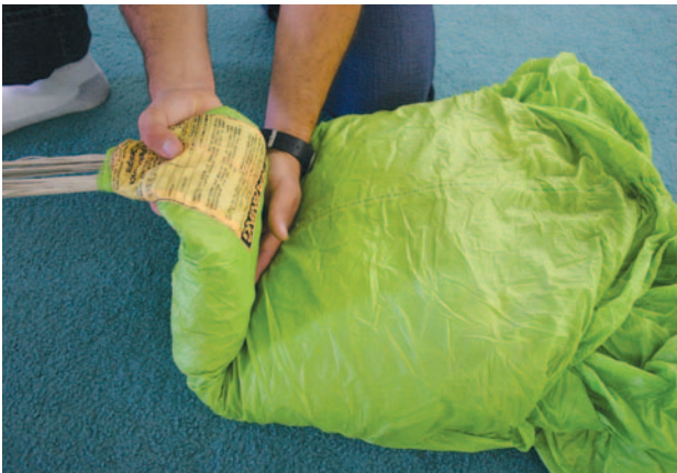
Figure 4-24. Make a short "S" fold at the slider end of the bundle.
