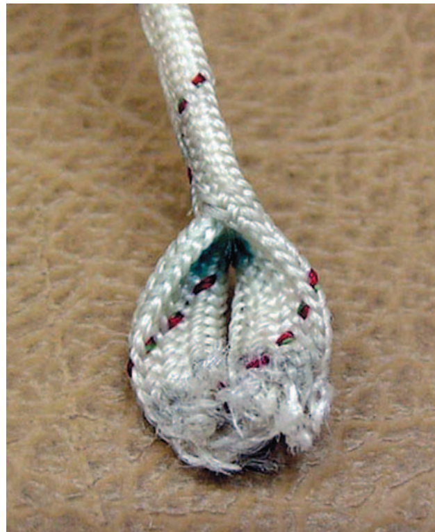
Figure 5-18. Worn closing loop.
