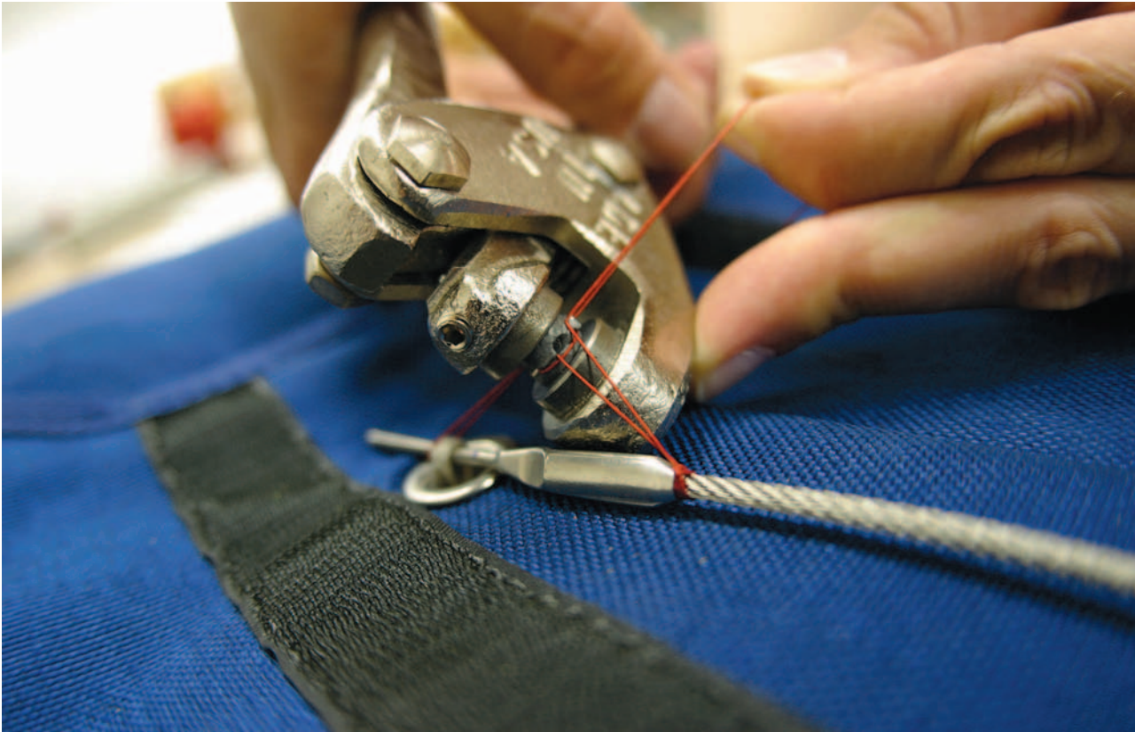
Figure 5-68. Compressing the seal.
