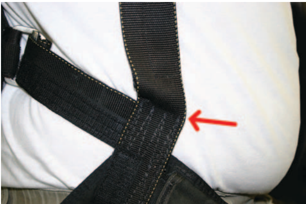
Figure 2-16. Standard harness junction warping.
