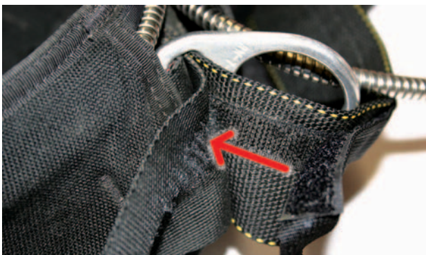
Figure 2-54. RSL Velcro® riser damage.
