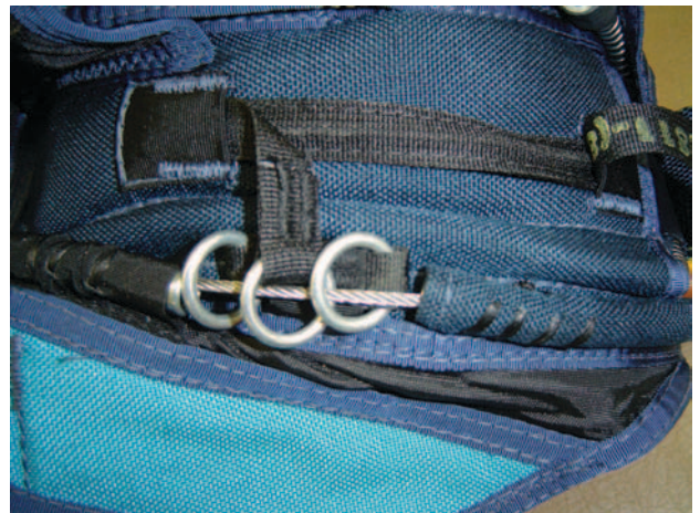
Figure 2-56. Ripcord cable routing thru rings.
