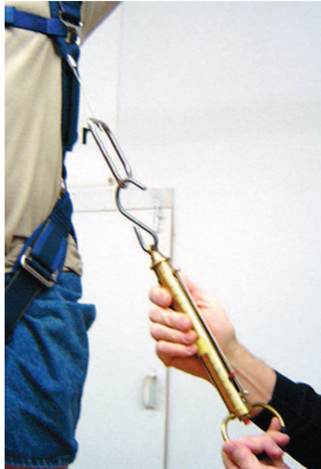
Figure 5-64. Ripcord pull test.
