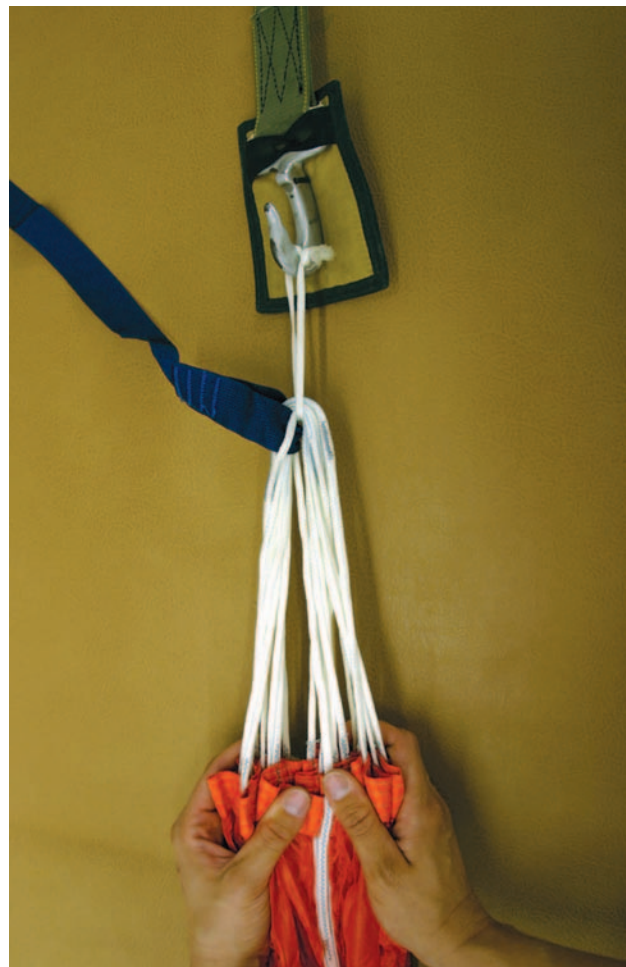
Figure 5-34. Straightening the canopy apex.
