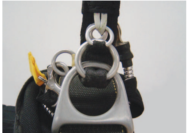
Figure 2-47. Single side RSL configuration.
