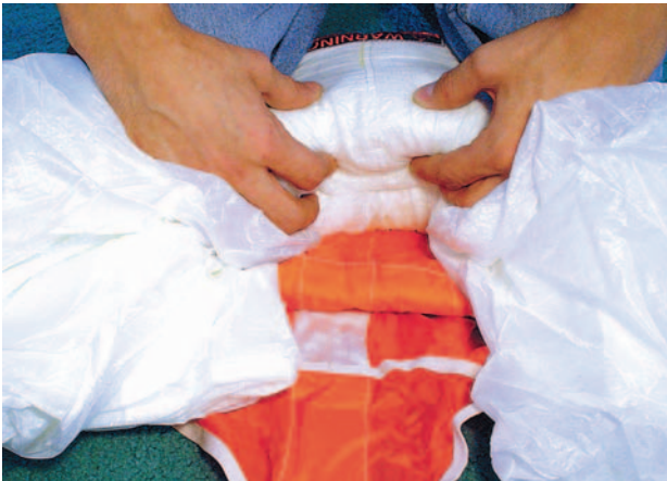
Figure 5-98. Gather and roll center seam fabric.
