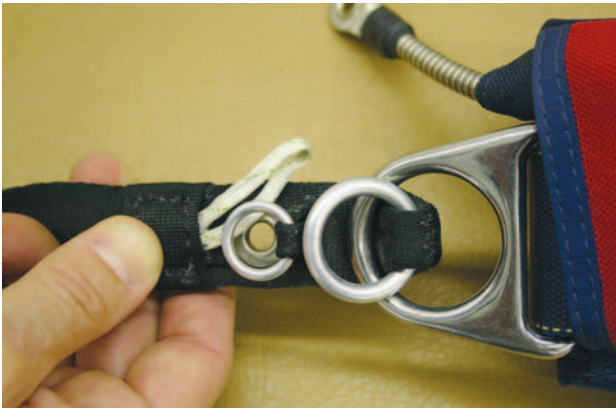
Figure 4-37. 3-ring middle thru large ring.
