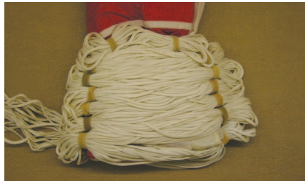
Figure 2-21. Type 3 deployment – Phantom canopy.
