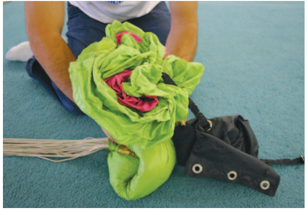
Figure 4-25. Fold the top of the canopy bundle back towards the lines for a second "S" fold.
