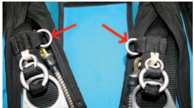
Figure 2-48. Dual side RSL configuration.
