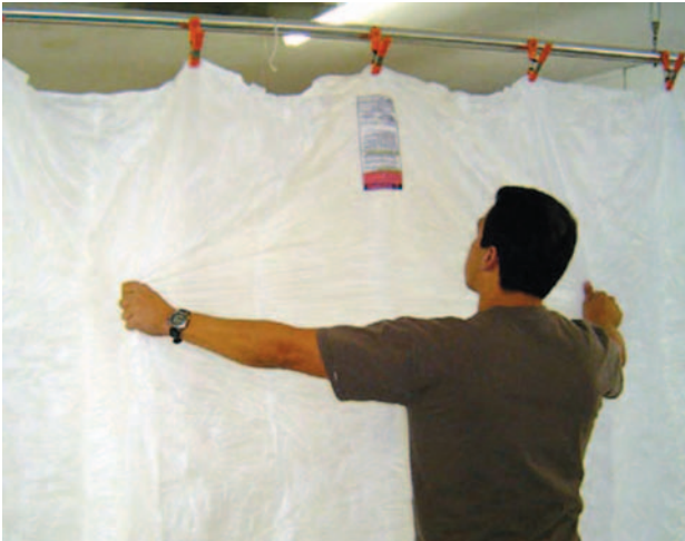
Figure 5-20. Ram-air canopy hanger—top skin inspection.
