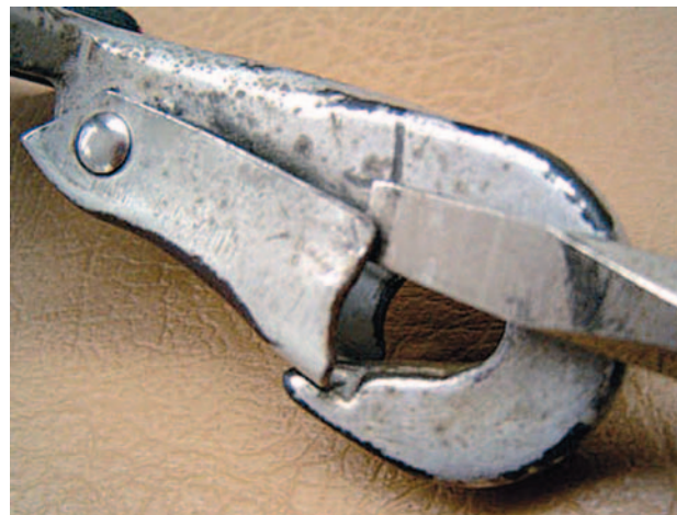
Figure 5-16. B-12 snap gate repair.
