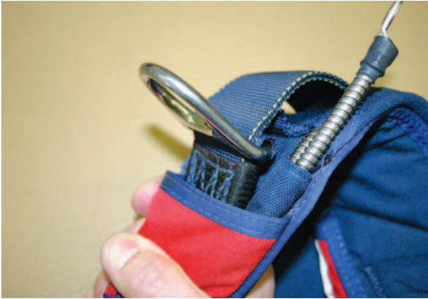
Figure 4-44. Harness 3-ring inspection.
