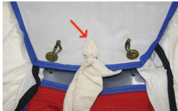
Figure 2-9. Square reserve hesitator loop configuration.
