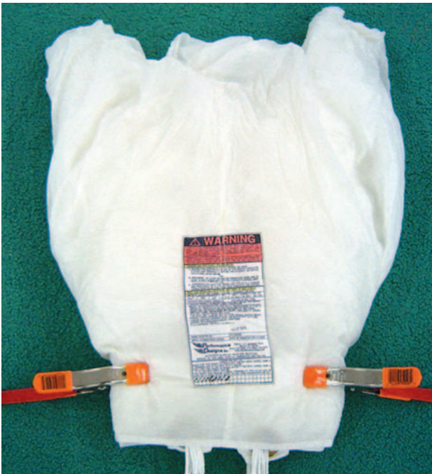
Figure 5-93. Wrap tail, two clamps.
