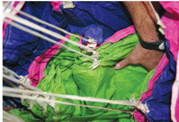
Figure 4-10. Separate and clear material between line groups.
