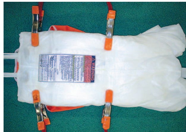
Figure 5-95. Bag positioned under canopy.
