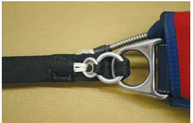
Figure 4-43. 3-ring finished from front.
