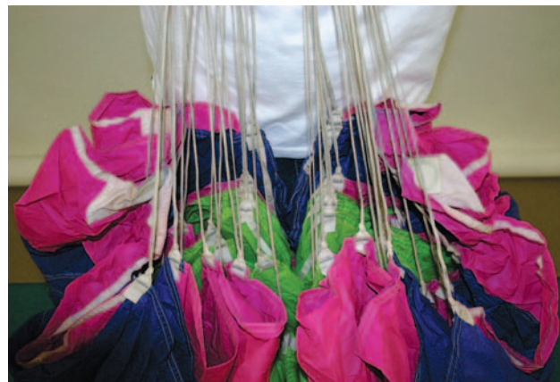
Figure 4-9. View from front with slider moved upward for clarity. Note how the attachment tapes of each line group fall together.
