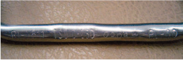
Figure 5-3. Reserve ripcord with TSO markings.
