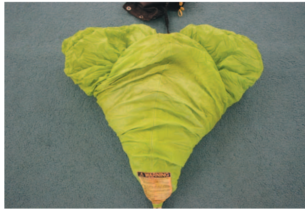
Figure 4-20. Triangular shape on the floor. Make sure the slider is securely wrapped in the tail.
