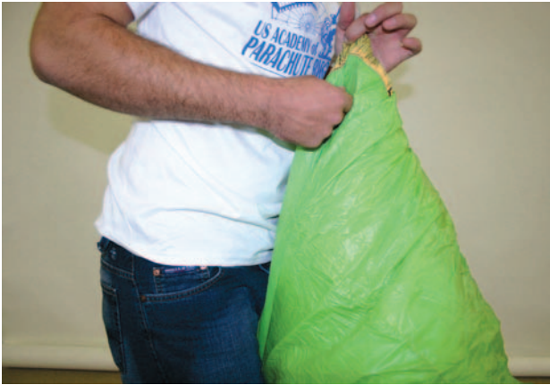
Figure 4-16. Hold the rolled tail between the legs and roll the upper material tightly against the lines.
