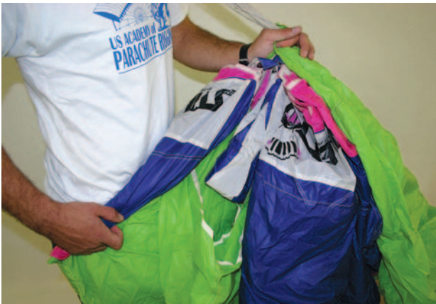
Figure 4-33. Rolling the nose of the canopy.
