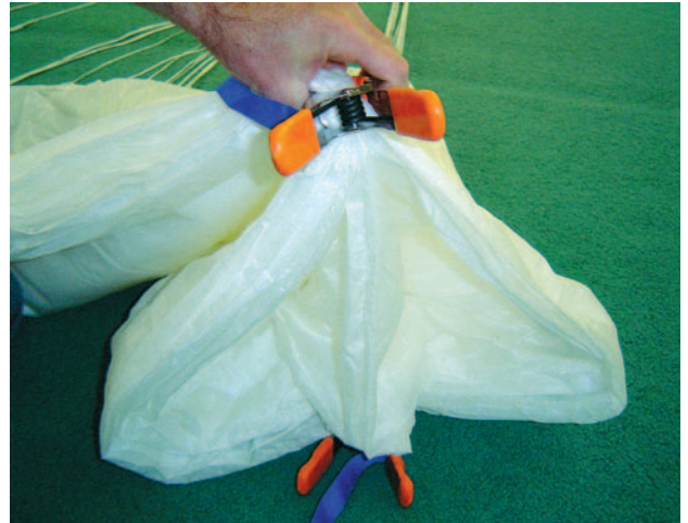
Figure 5-79. Lower "B" clamp to "A" clamp, spreading the cells.
