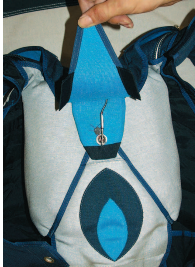
Figure 5-113. Close flap #4 and insert ripcord pin.
