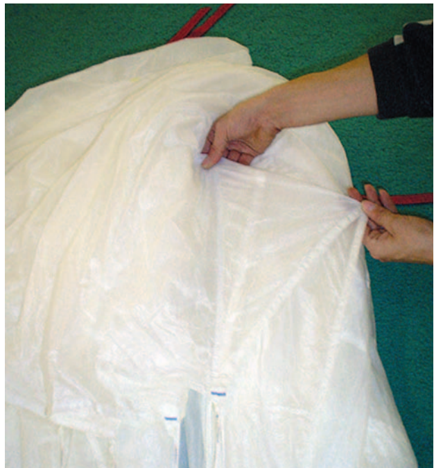
Figure 5-86. Pull stabilizer taut.
