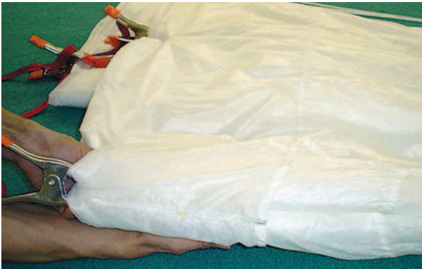
Figure 5-77. Smooth panels under "A" lines.
