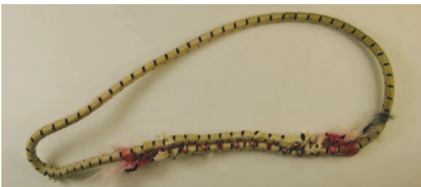
Figure 2-30. Bad Safety Stow®.
