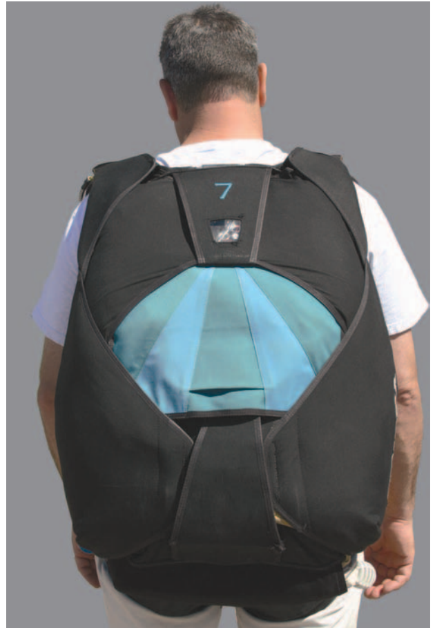
Figure 2-7. Tandem container system.
