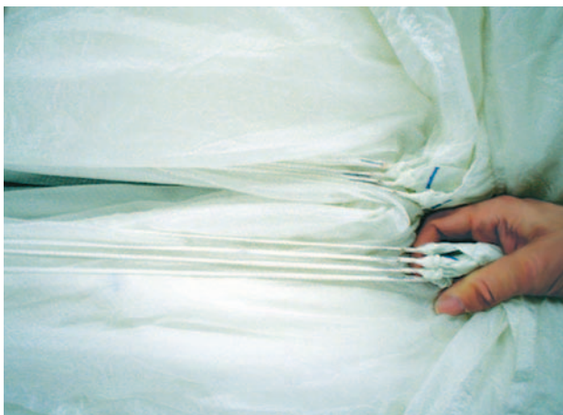
Figure 5-88. Lines are taut in the center.
