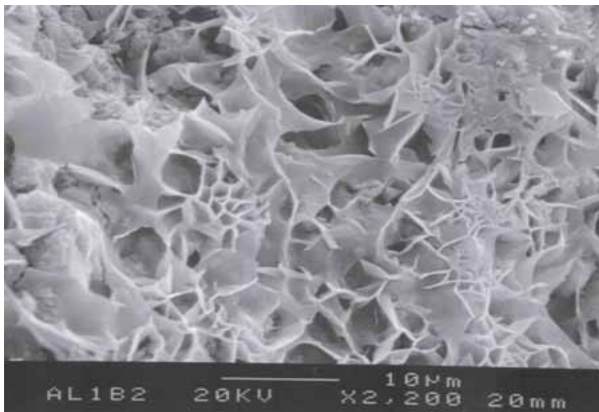
Figure 3-11. Crystalline lamellar gel at the surface of aggregate.
