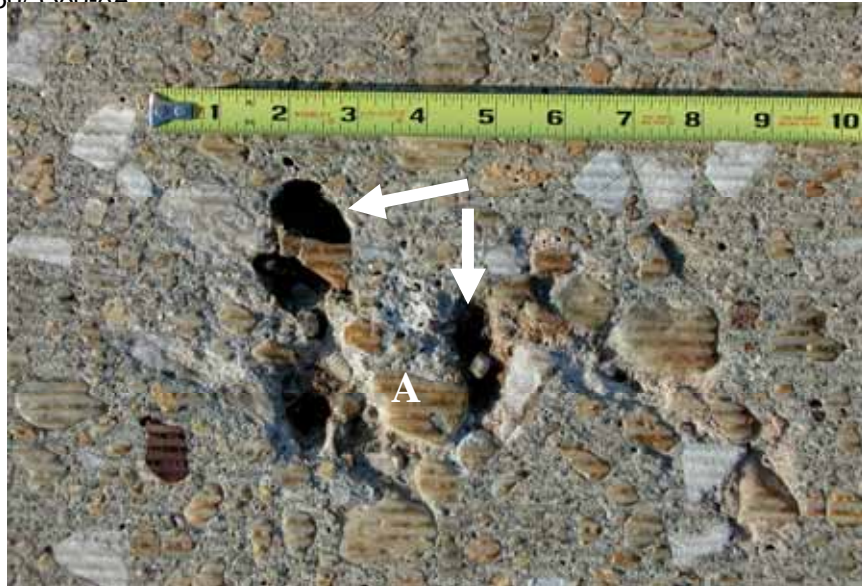
Figure 2-7. Several aggregate particles (A) have been dislodged (→) along with some neighboring paste.
