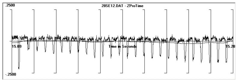
The figure is a close order (0.20 seconds) laser profile of a grooved pavement surface.
