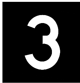
Figure 15. Runway Distance Remaining Sign
