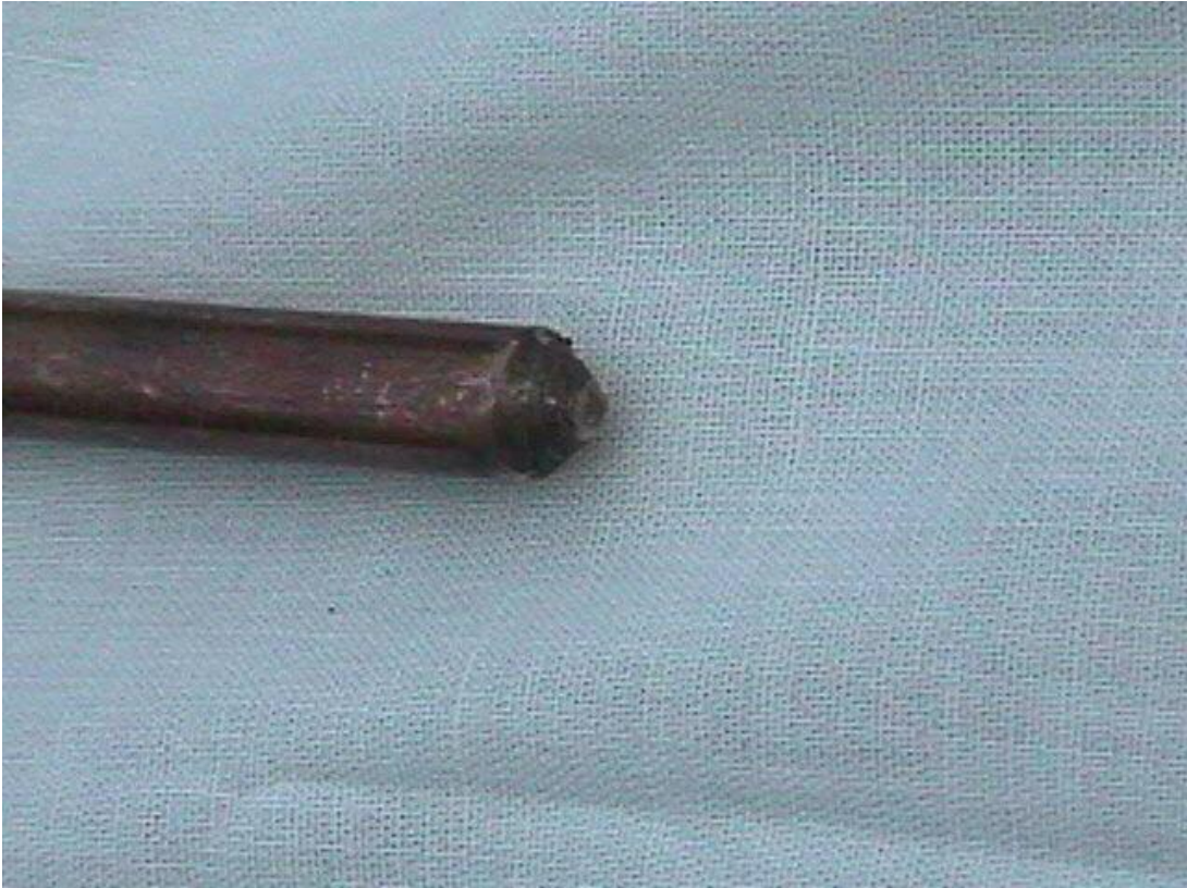
No. 5 : We can see the cone shape end of the rod with which the rod will be grounded.
