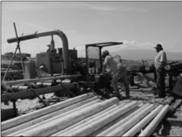
Mill workers remove bark from small-diameter trees.
