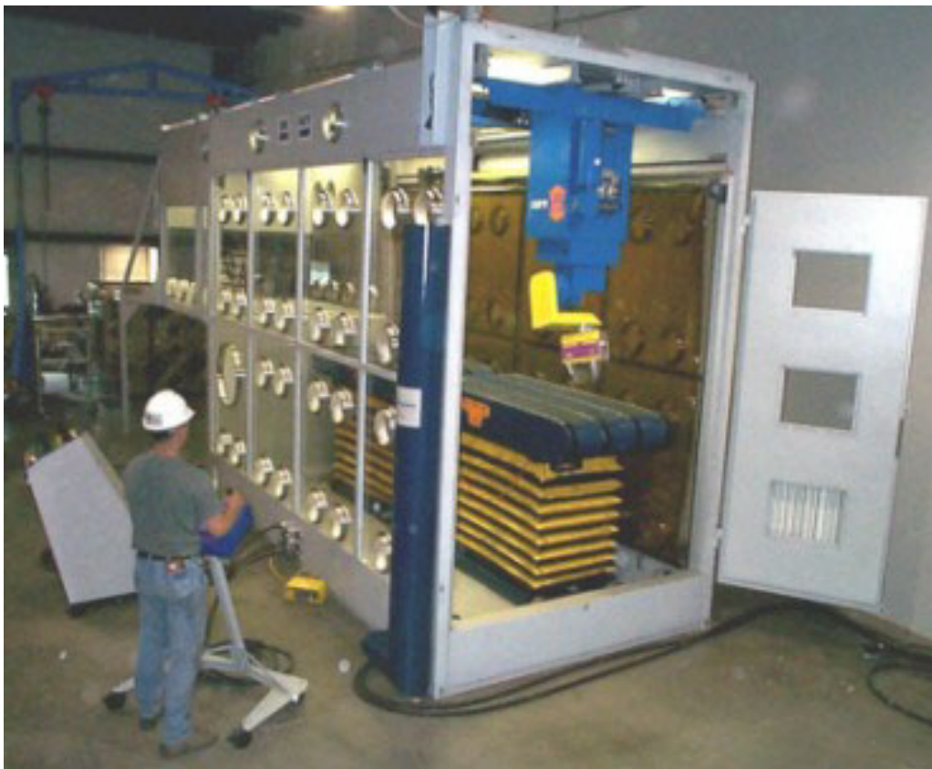
Figure 11. Example of a remotely operated dismantling system and inspection station.
