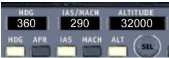
Figure 4. Our autopilot, showing its three “dimensions” of heading, indicated airspeed, and altitude . Each triplet can comprise one “maneuver” inside a state space.
