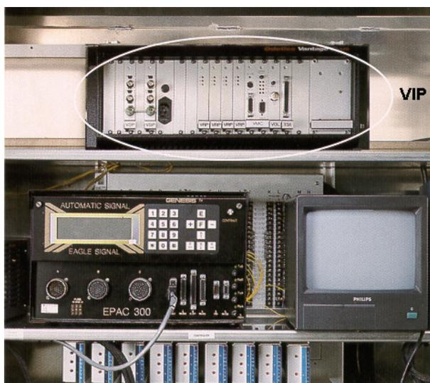
Figure 2-51. Video image processor installed in a roadside cabinet (Photograph courtesy of Iteris, Anaheim, CA).
