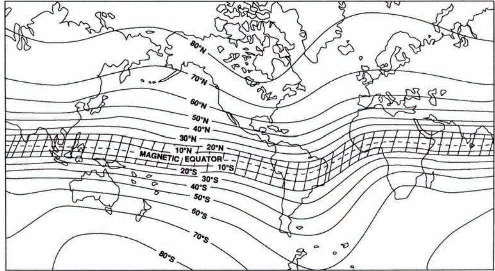
Figure 2-41. Equatorial belt showing where Earth's magnetic field is too small for deployment of simple vertical axis magnetometers between 20 degrees north and 20 degrees south of the Equator.
