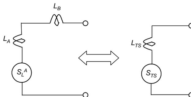
Figure 2-15. Equivalent total inductance from two inductive loops in series.
