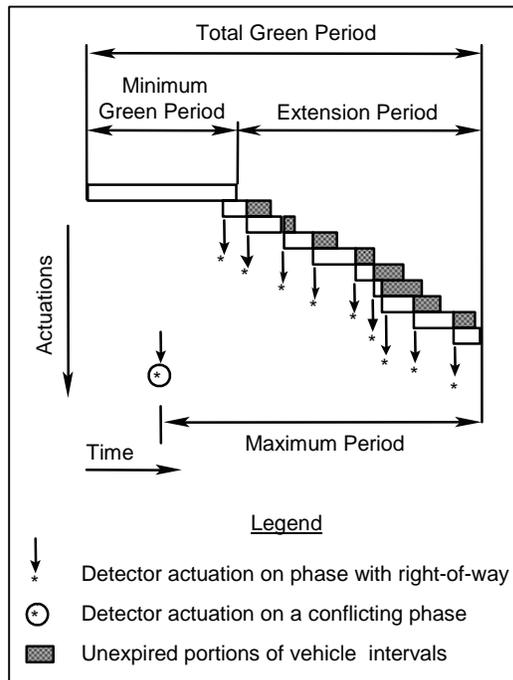
Figure 4-1. Actuated controller green phase intervals.
