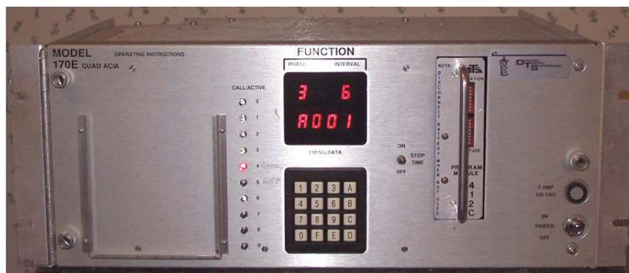
Figure 2-36. Model 170 controller (Photograph courtesy of Lawrence A. Klein).
