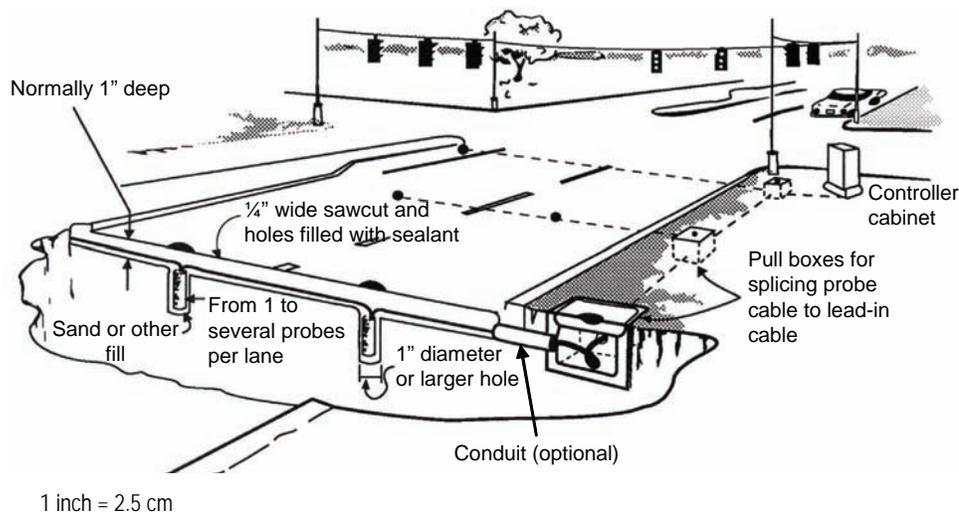
Figure 2-39. Magnetic sensor installation.
