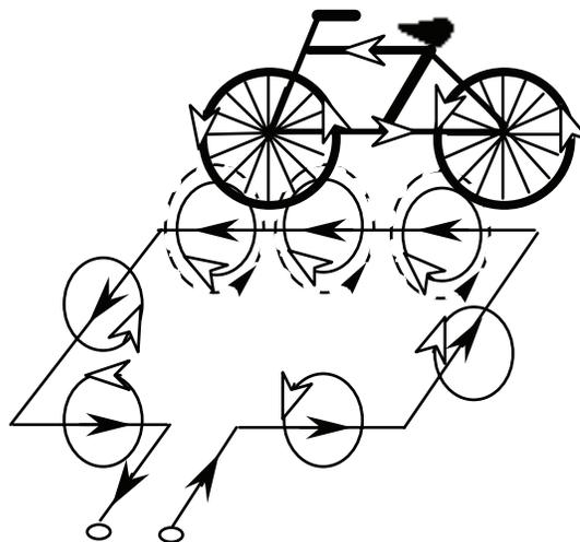
Figure 2-9. Bicycle detection showing induced eddy currents. The black arrows represent the current flow in the loop wire and the white arrows the induced flux.
