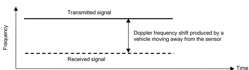
Figure 2-57. Constant frequency waveform.
