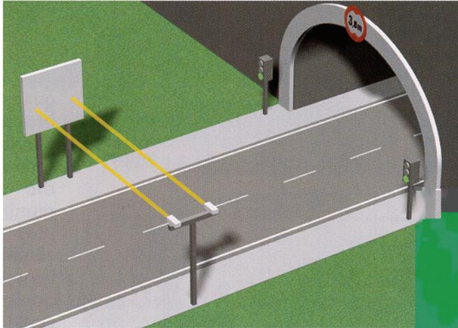
Figure 3-29. Overheight sensor configuration (Picture courtesy of MBB SensTech, Munich, Germany).
