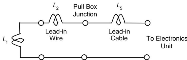
Figure 2-18. Equivalent single loop electrical circuit.
