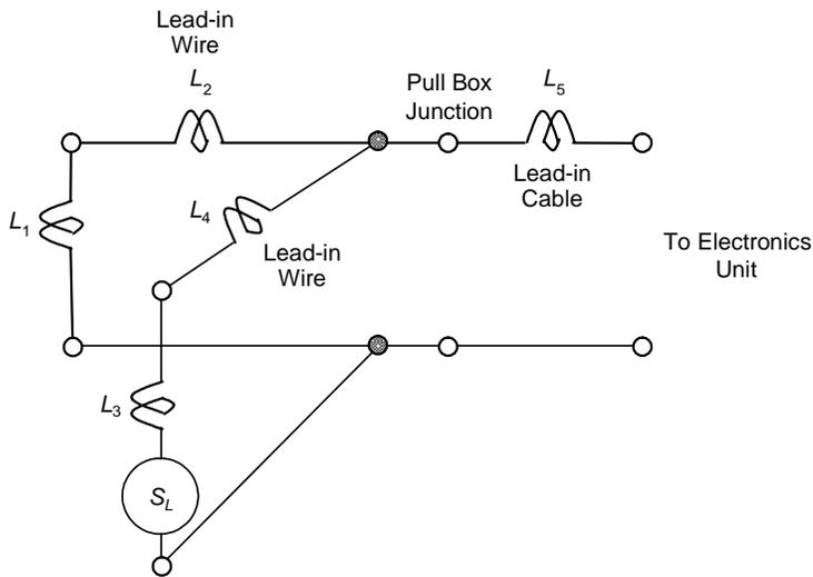
Figure 2-22. Equivalent electrical circuit for two loops connected in parallel to a pull box and electronics unit.
