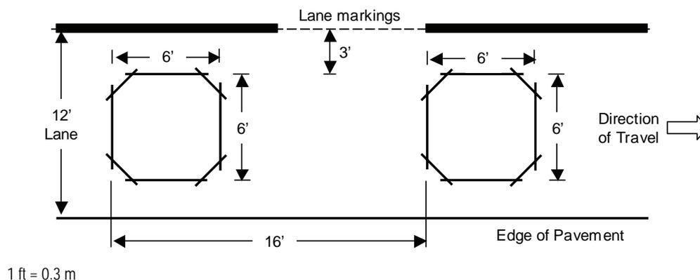
Figure 3-1. Vehicle speed measurement using two inductive-loop detectors placed a known distance apart.
