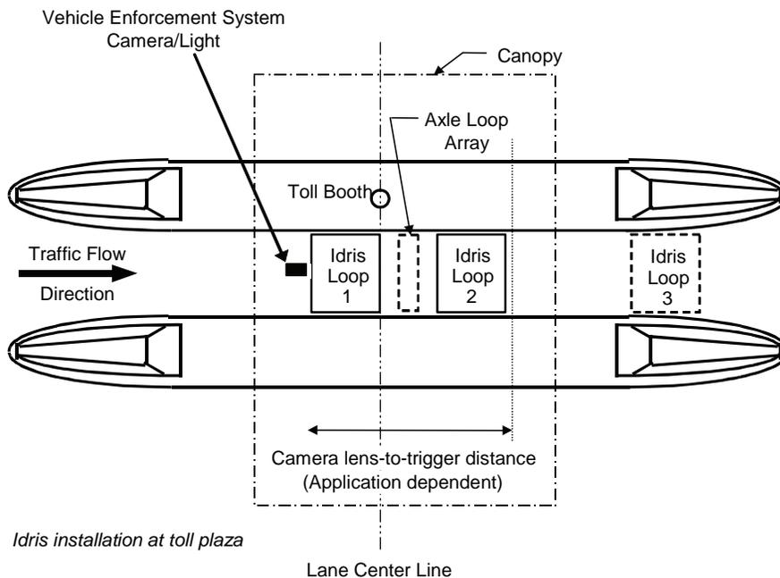
Figure 2-30. Axle location and vehicle classification using an array of inductive loops
