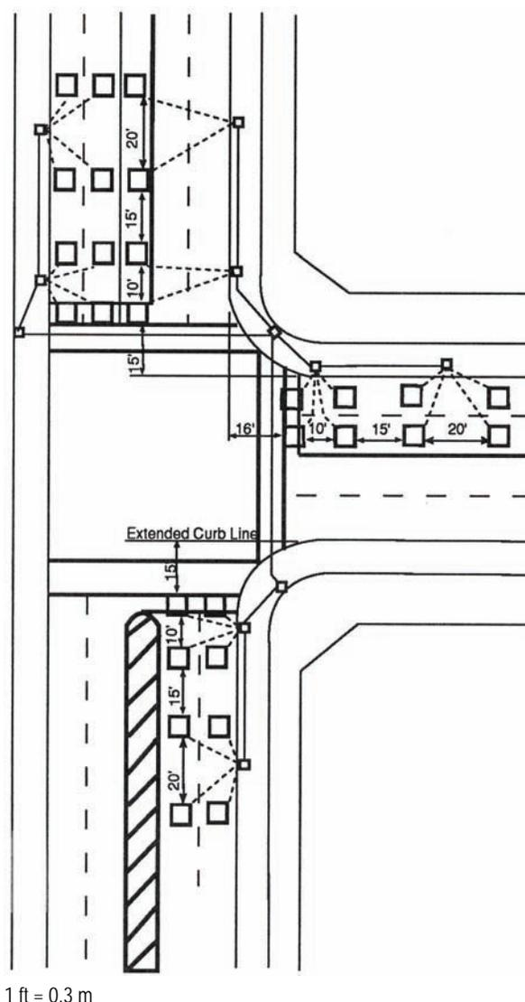
Figure 4-13. PennDOT short inductive-loop configurations.
