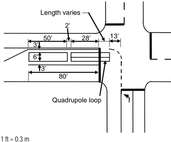
Figure 4-15. Left turn detection inductive-loop configuration used by IDOT.
