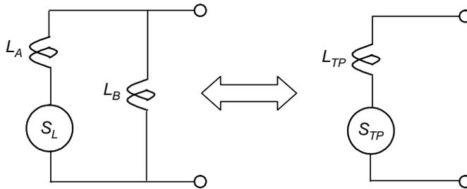
Figure 2-16. Equivalent total inductance from two inductive loops in parallel.
