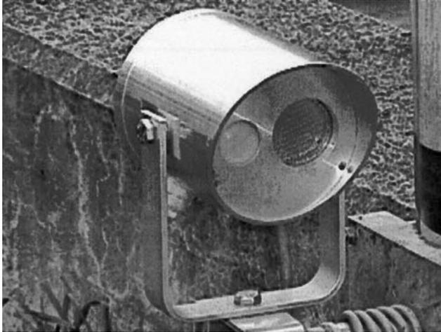
ASIM DT 272 Passive infrared-ultrasonic sensor.
