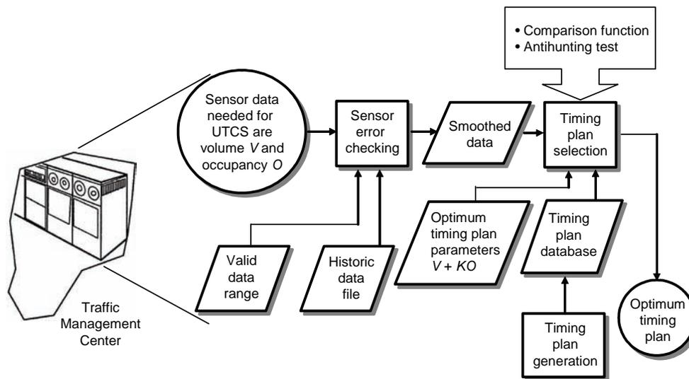
Figure 3-6. UTCS timing plan selection procedure.
