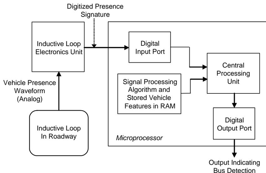
Figure 3-18. Inductive-loop detection system for transit vehicles.
