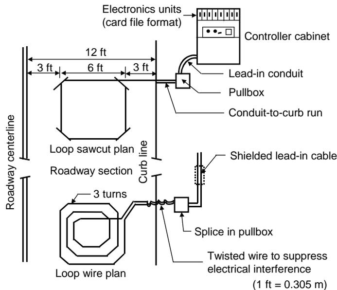
Figure 1-4. Inductive-loop installation example.
