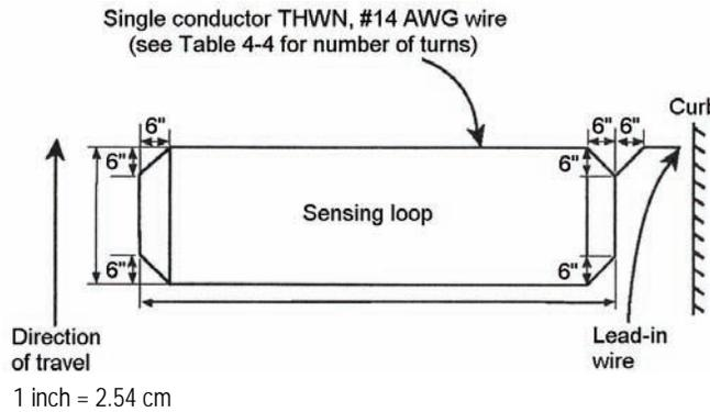
Figure 4-14. Wide inductive-loop detector layout.
