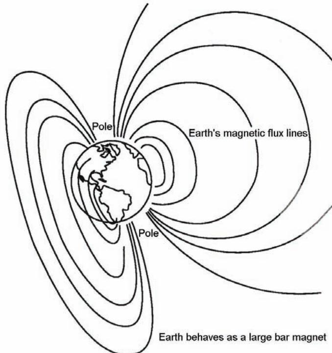
Figure 2-40. Earth's magnetic flux lines.
