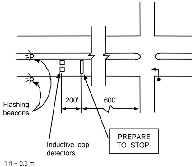
Figure 4-8. PREPARE TO STOP inductive-loop detector system.
