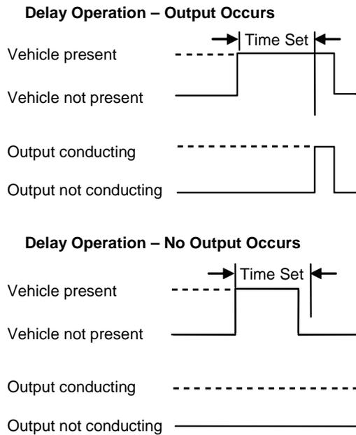
Figure 2-34. Delay operation.
