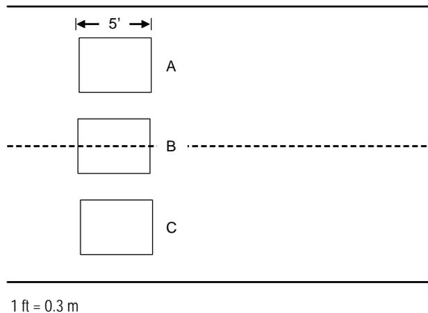
Figure 3-27. Three-loop layout for counts.
