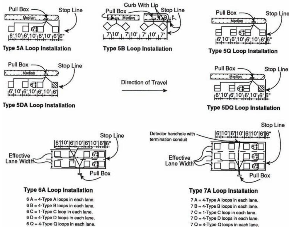
Figure 4-12. Caltrans standard sequential inductive-loop configurations.
