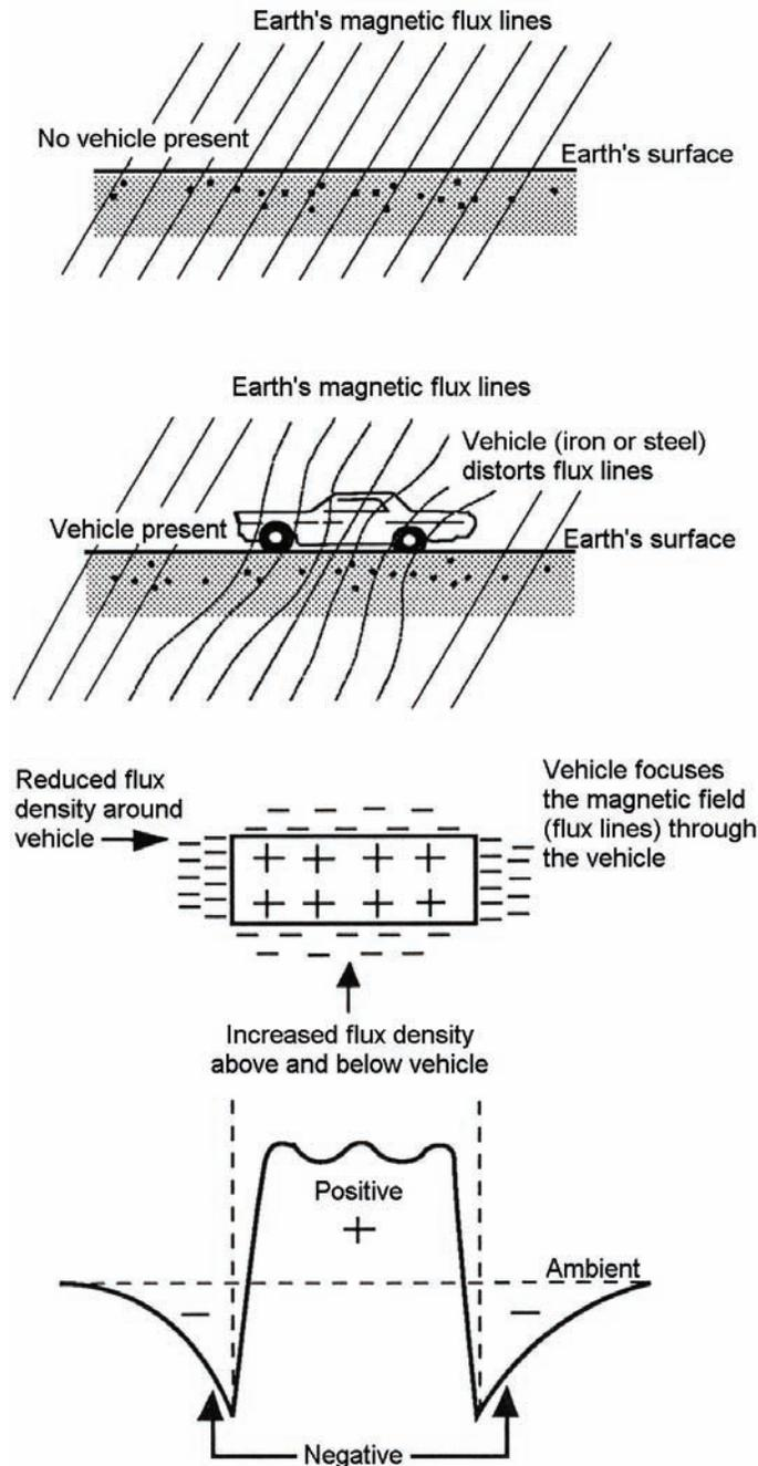
Figure 2-42. Distortion of Earth's quiescent magnetic field by a ferrous metal vehicle.
