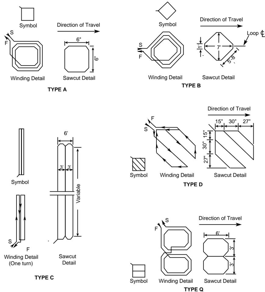
Figure 4-10. Caltrans-specified loop shapes.
