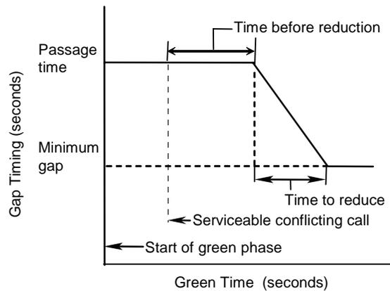
Figure 4-3. NEMA gap reduction procedure.
