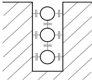
Figure 2-4. Capacitive coupling between the loop wires themselves and the sawcut slot sidewalls.
