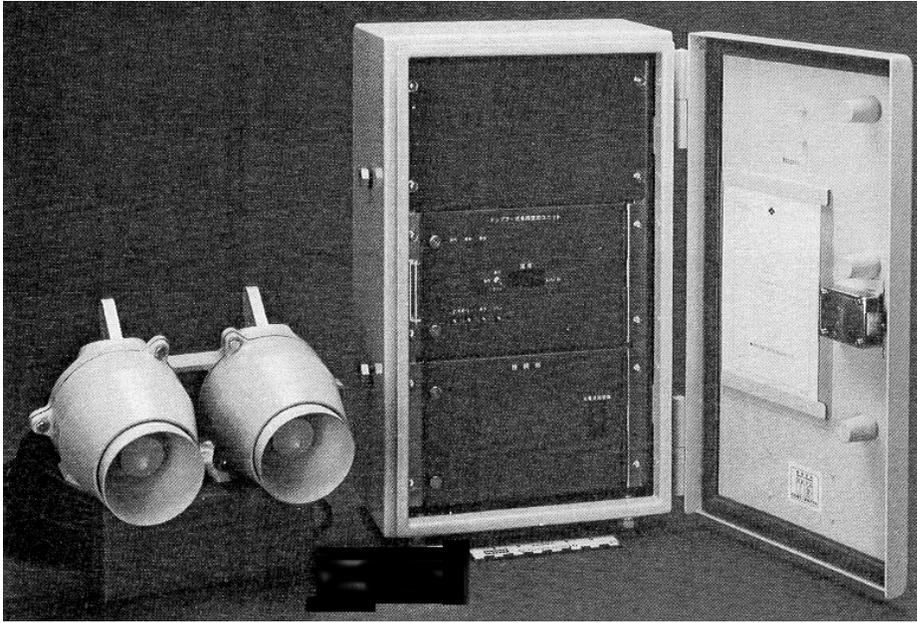
Figure 2-71. Speed-measuring RDU-101 Doppler ultrasonic sensor (manufactured by Sumitomo Electric, Japan) with separate transmitting and receiving transducers, as shown in the left portion of the figure. The cabinet on the right contains the electronic systems needed to supply power and control signals to the transducers, receive the data, and interface with the highway infrastructure.
