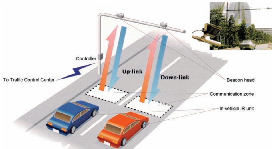
Figure 2-64. Active infrared sensor installed for transmitting traffic conditions to motorists
