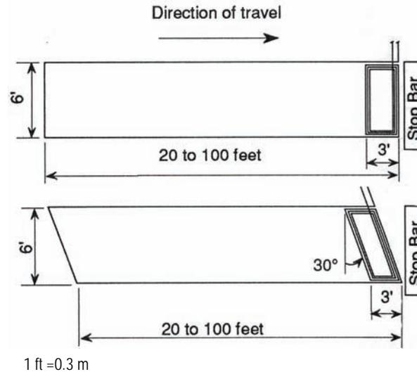
Figure 4-27. Long loop with powerhead.
