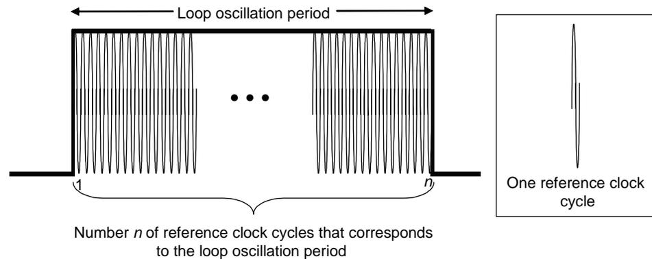
Figure 2-27. Measurement of inductive-loop oscillation period by a reference clock (Source: L.A. Klein, *Sensor Technologies and Data Requirements for ITS* (Artech House, Norwood, MA, 2001)).
