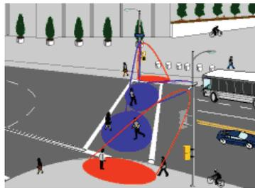
(b) Microwave radar sensing
