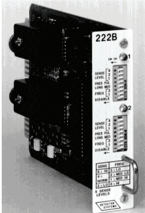
Figure 2-32. Two-channel card rack mounted electronics unit.
