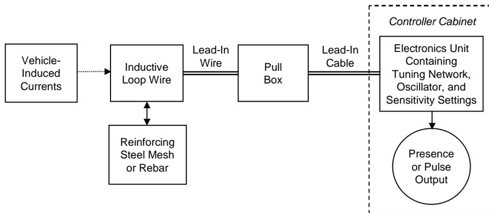
Figure 2-1. Inductive-loop detector system (notional).
