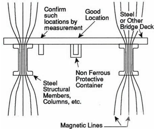
Figure 4-34. Typical installation of magnetometers on a bridge deck.
