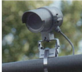
Siemens Eagle PIR-1 sensor. Performs vehicle counting, stop line presence detection, occupancy detection, and queue detection. (Photograph courtesy of Siemens ITS, Austin, TX).
