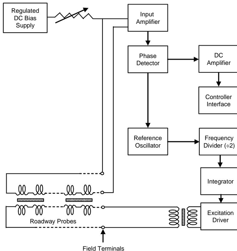
Figure 2-44. Magnetometer sensor probe and electronics unit equivalent electrical circuit.
