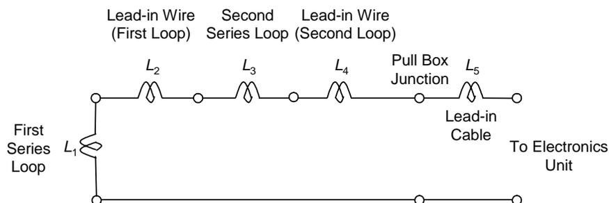
Figure 2-20. Equivalent electrical circuit for two loops connected in series to a pull box and electronics unit.
