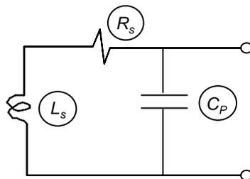
Figure 2-5. Equivalent electrical circuit for an inductive loop with capacitive coupling to the sidewalls of a sawcut slot.
