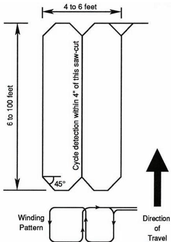
Figure 4-23. Quadrupole loop configuration.
