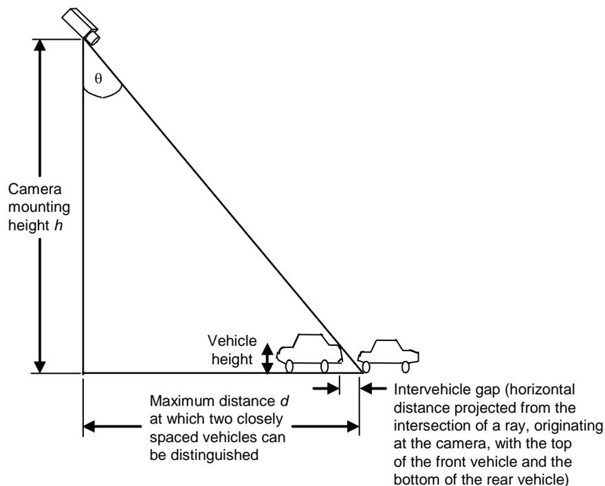
Figure 2-55. Distinguishing between two closely spaced vehicles (source: L.A. Klein, *Sensor Technologies and Data Requirements for ITS* (Artech House, Norwood, MA, 2001)).
