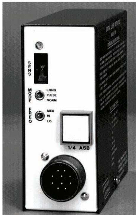
Figure 2-31. Shelf-mounted NEMA electronics unit.
