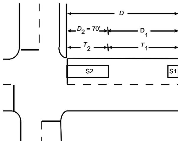
Figure 4-21. Extended call inductive-loop detector system.
