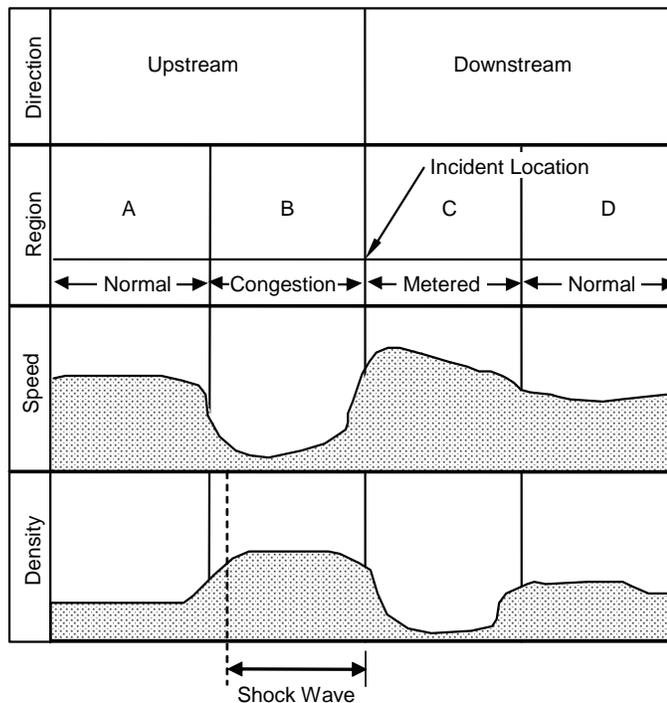
Figure 3-7. Traffic flow characteristics during an incident (source: *Intelligent Vehicle Highway Systems: The State of the Art*, prepared for Massachusetts Department of Highways (JHK and Associates, New York, NY, March 1993)).
