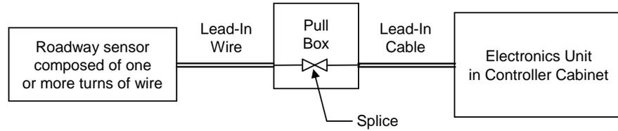
Figure 1-3. Inductive-loop detector system.
