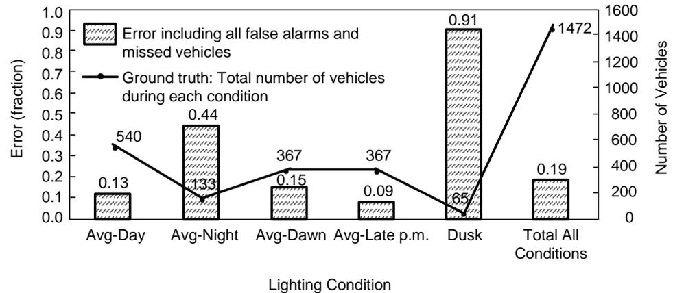
Figure 2-54. VIP vehicle count errors under varying illumination conditions. Low camera sensitivity, improper focal length of lens, low camera resolution, nonideal camera mounting height, inadequate video signal, and lack of sun shade contributed to degraded performance (source: *Traffic Surveillance and Detection Technology Development: Phase II and III Test Results*, Troy, MI, JPL Pub. D-15779 (California Institute of Technology, Jet Propulsion Laboratory, Pasadena, CA, May 1998)).
