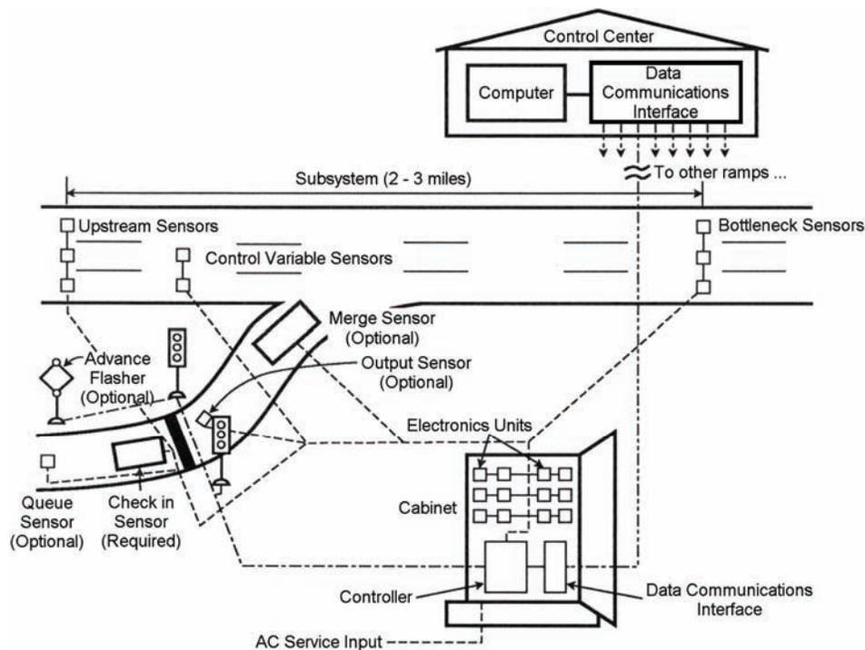
Figure 3-10. Conceptual coordinated traffic responsive ramp control system.
