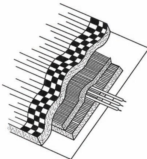
Figure 2-24. Five-layer temporary open loop detector configuration.
