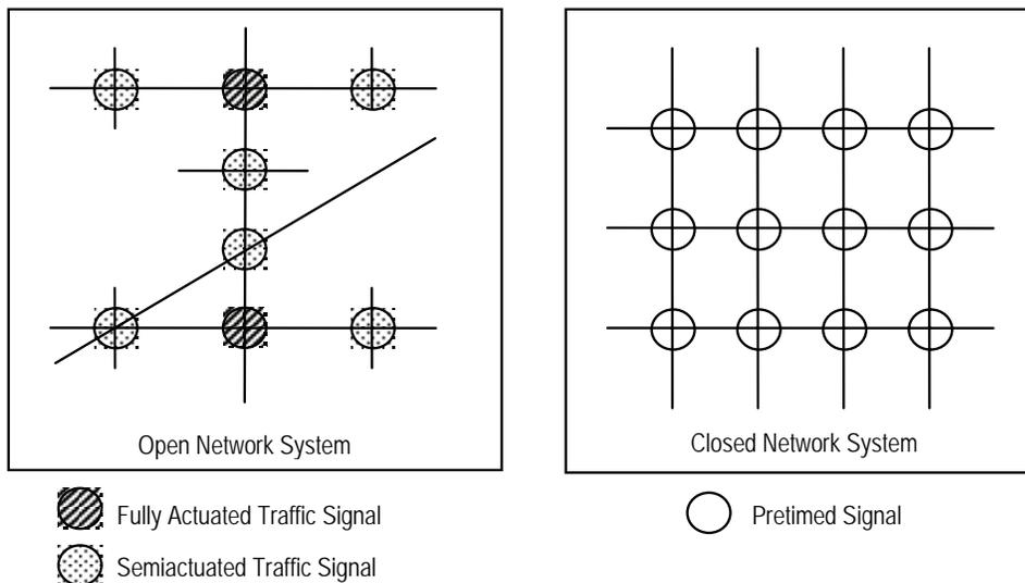
Figure 3-5. Arterial open network and surface street closed network traffic signal configurations typical of those found in interconnected intersection control.
