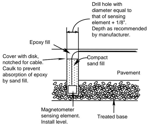
Figure 4-33. Conceptual magnetometer sensor installation.
