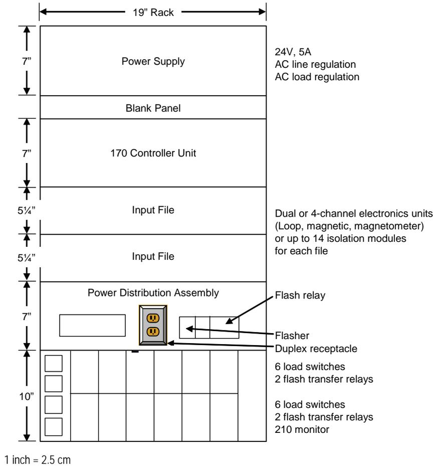
Figure 2-37. Type 170 cabinet layout (California).
