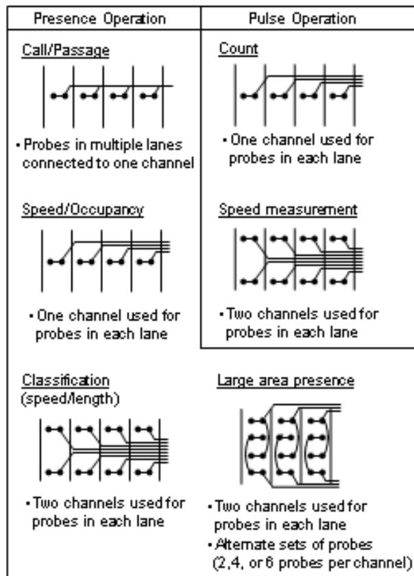
Figure 4-36. Magnetometer-probe placement in support of several data-gathering functions.
