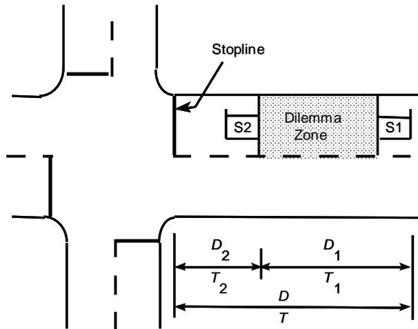
Figure 4-20. Green extension system using two inductive-loop detectors.
