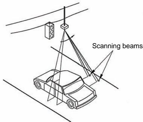
Figure 1-9. Scanning infrared laser radar two-beam pattern across a traffic lane (Drawing courtesy of Schwartz Electro-Optics, now OSI Laserscan, Orlando, FL).
