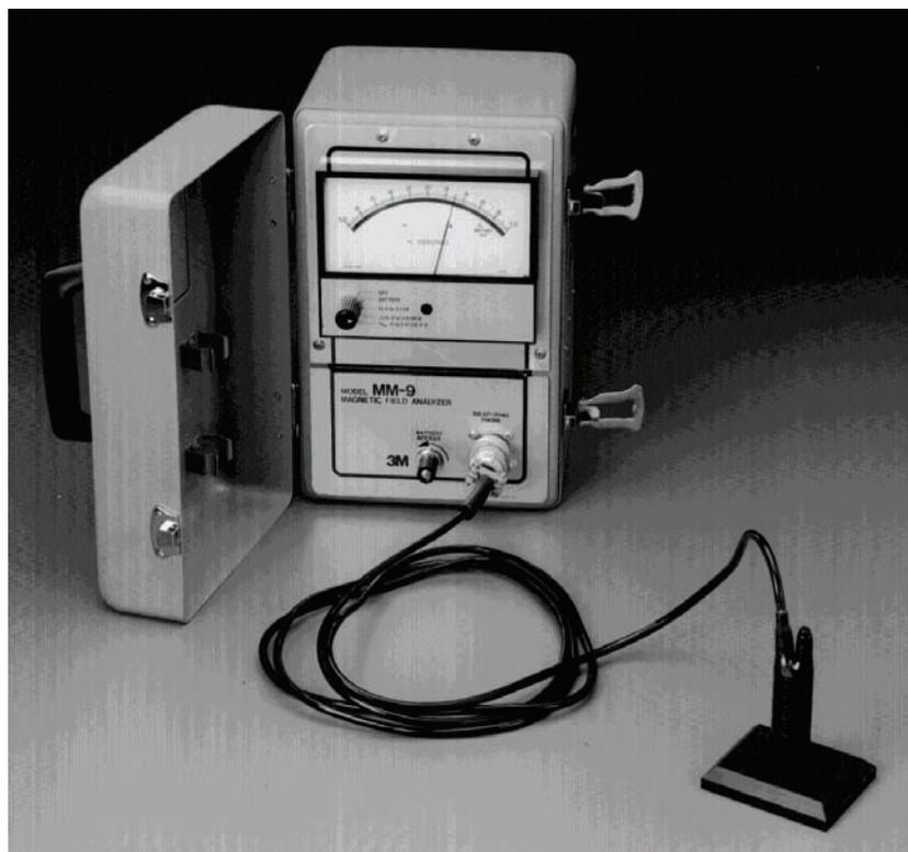
Figure 4-35. Magnetic field analyzer.
