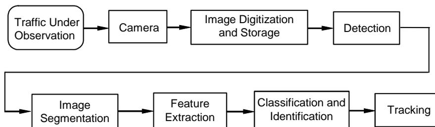
Figure 2-52. Conceptual image processing for vehicle detection, classification, and tracking.
