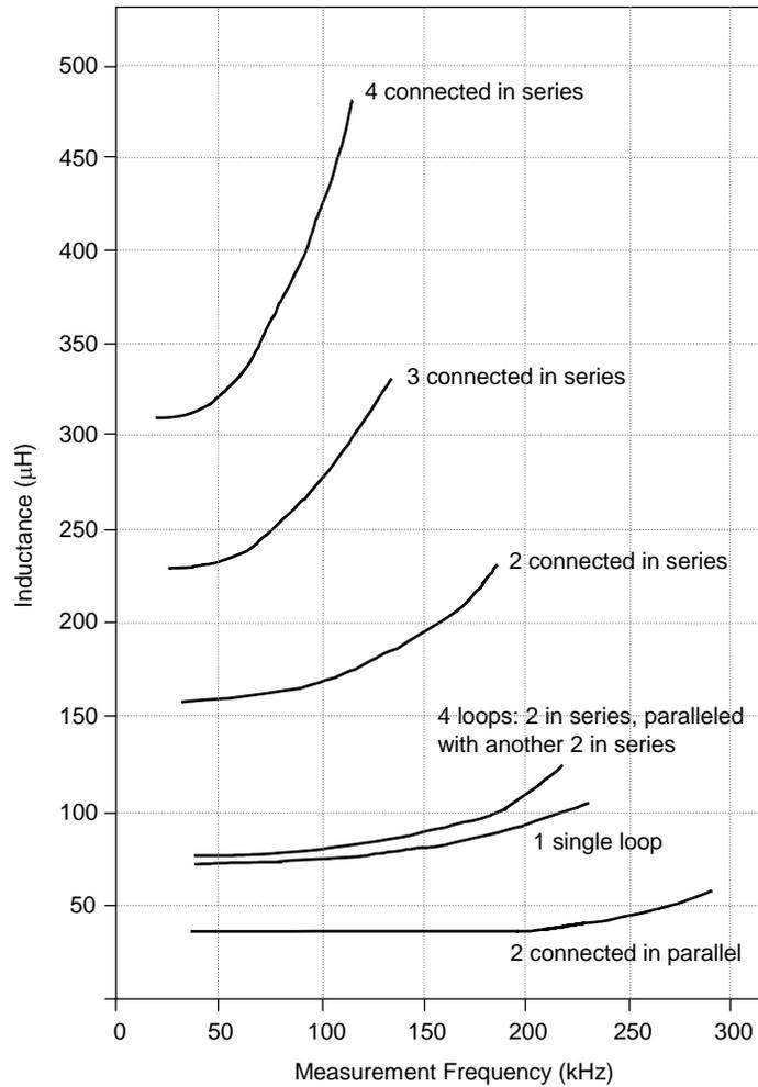
Figure 2-6. Average values of loop inductance vs. measuring frequency for series, parallel, and series-parallel connections of 6- x 6-ft (1.8- x 1.8-m) inductive loops. The plots represent curve fits to the measured data.
