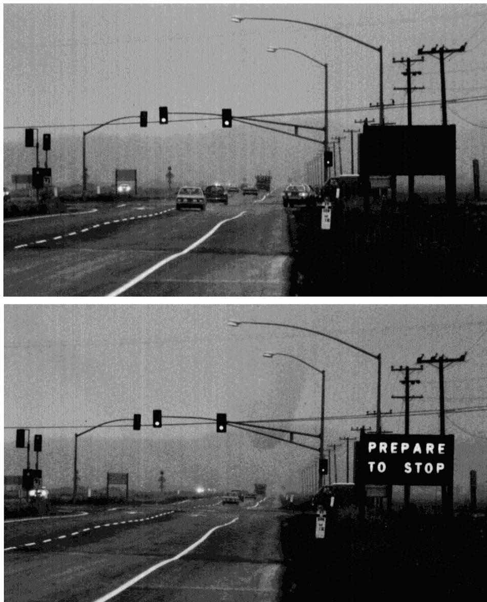
Figure 4-7. PREPARE TO STOP sign on an arterial in nonilluminated and illuminated states.
