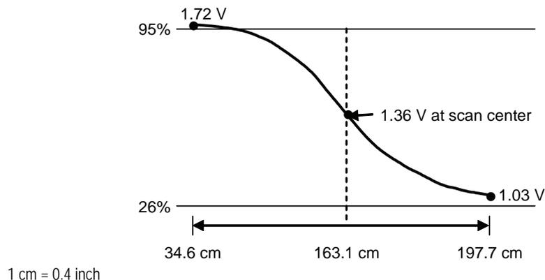
Figure 3-33. Output voltage generated by passive lane positioning sensor.
