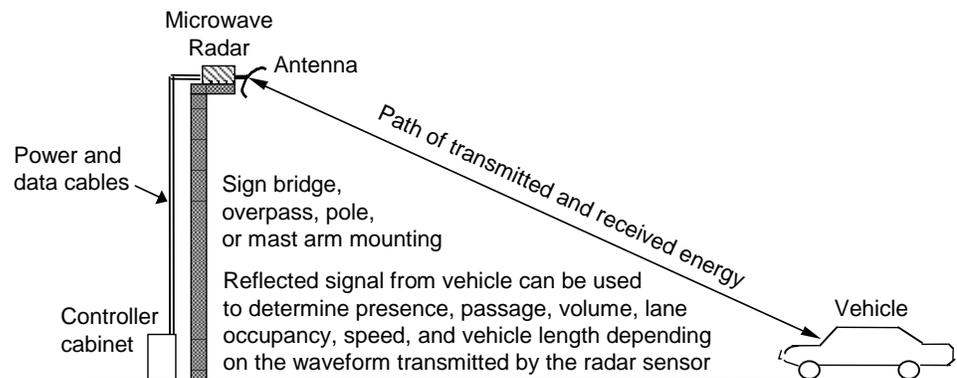
Figure 1-7. Microwave radar operation.
