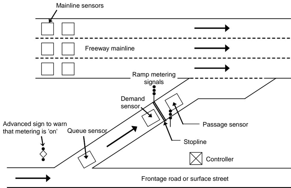
Figure 3-9. Conceptual ramp metering sensor and roadway configurations.
