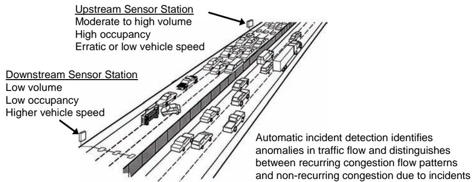
Figure 3-8. Freeway incident detection scenario.
