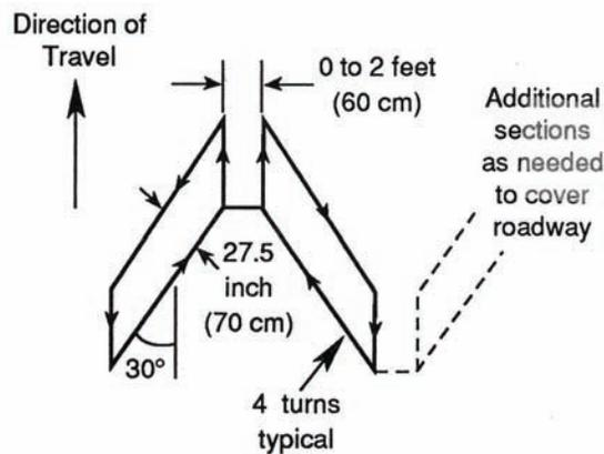
Figure 4-26. Chevron-loop configuration.
