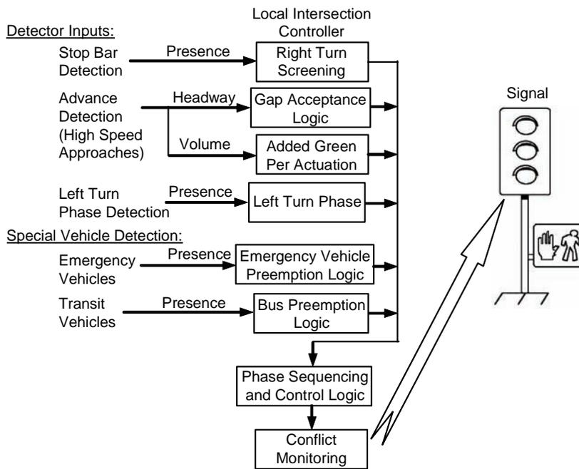
Figure 3-3. Data processing at an intersection with isolated intersection control.
