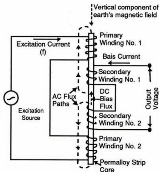
Figure 2-43. Magnetometer sensor electrical circuit (notional).
