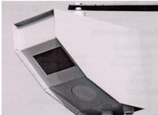
ASIM DT 281 Passive infrared-CW Doppler microwave radar sensor.
