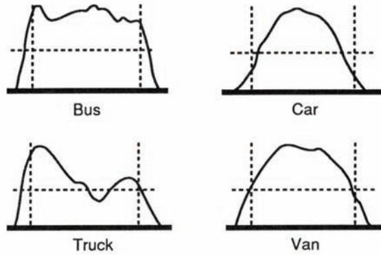
Figure 3-19. Representative vehicle signatures obtained from loops excited by high frequency signals from specialized electronics units.
