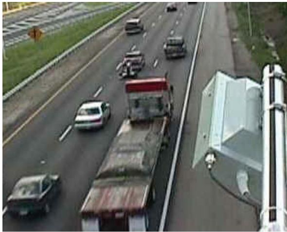
SAS-1 acoustic sensor (Photograph courtesy of SmarTek Systems, Woodbridge, VA).
