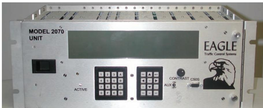
Figure 2-38. Model 2070 controller. The 2070 ATC controller is manufactured by Econolite, Eagle, Naztec, Safetran, GDI Communications, and McCain Traffic Supply at present.
