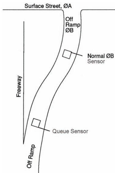
Figure 4-32. Queue discharge system.
