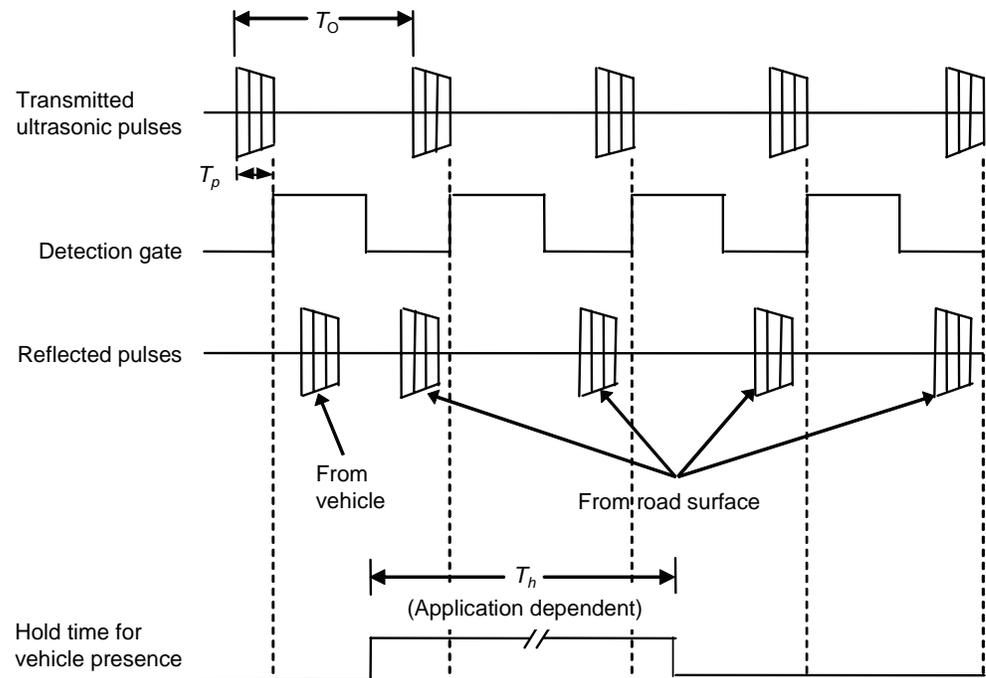
Figure 2-72. Operation of range-measuring ultrasonic sensor.
