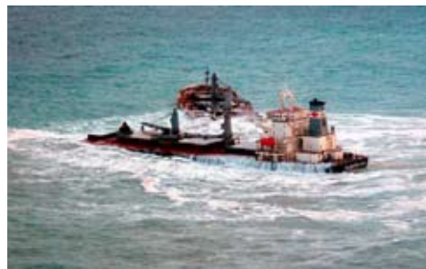
The Selendang Ayu broken in two and leaking oil off the coast of Unalaska, AK.
