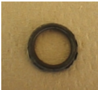
Figure 5 Inner O-ring Showing Wear
