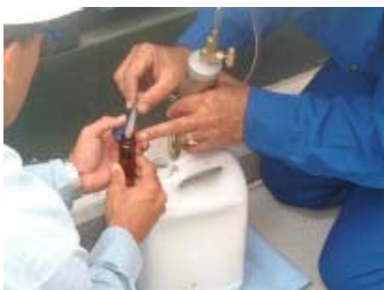
Figure 4. Transformer Sampling performed at SMHS and TI
