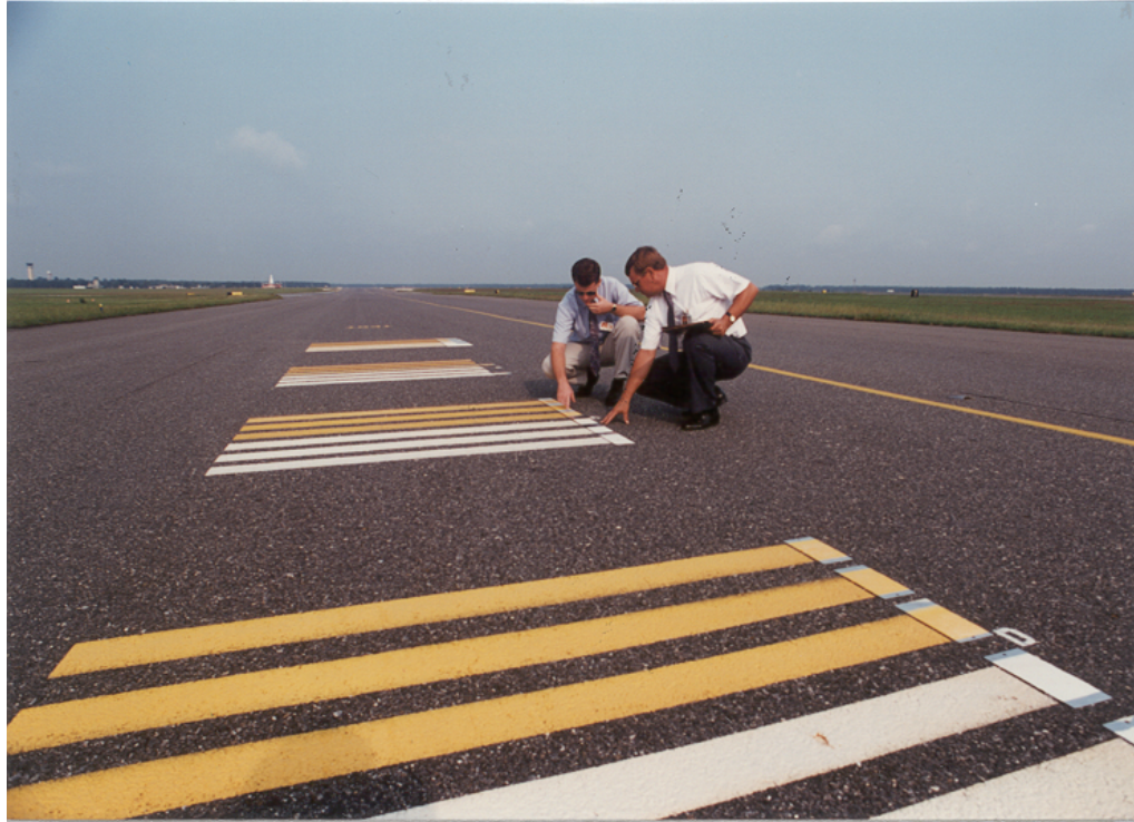
FIGURE A-16. EXAMINING DRAWDOWNS FOR COLOR RETENTION
