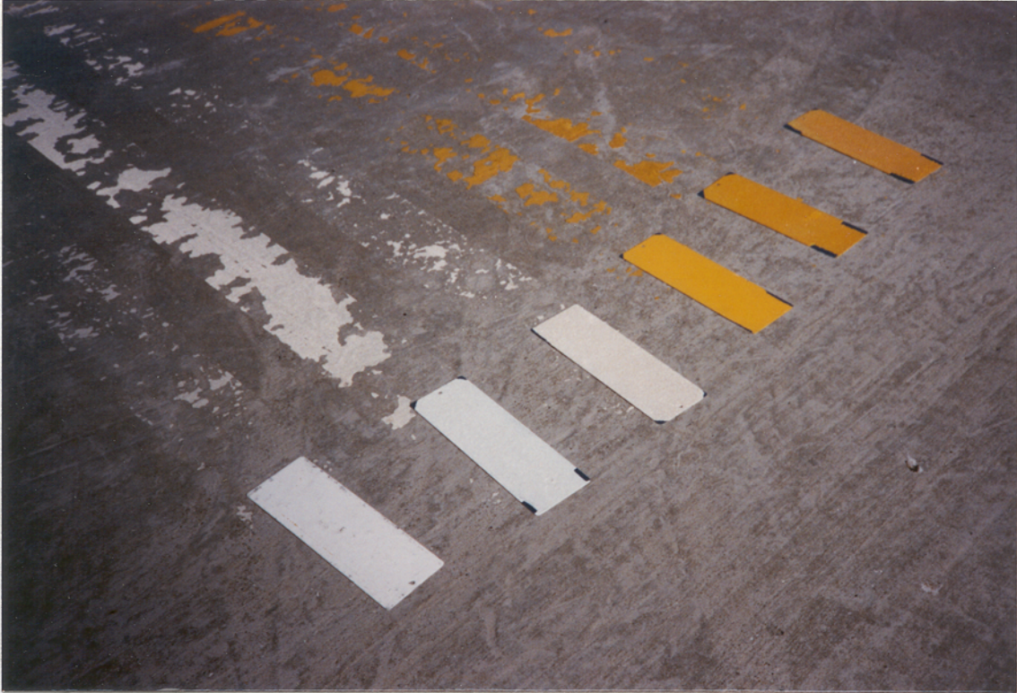
FIGURE A-30. WATER-BORNE NO. 1 TAXIWAY TEST STRIPE AFTER 1 YEAR - PITTSBURGH
