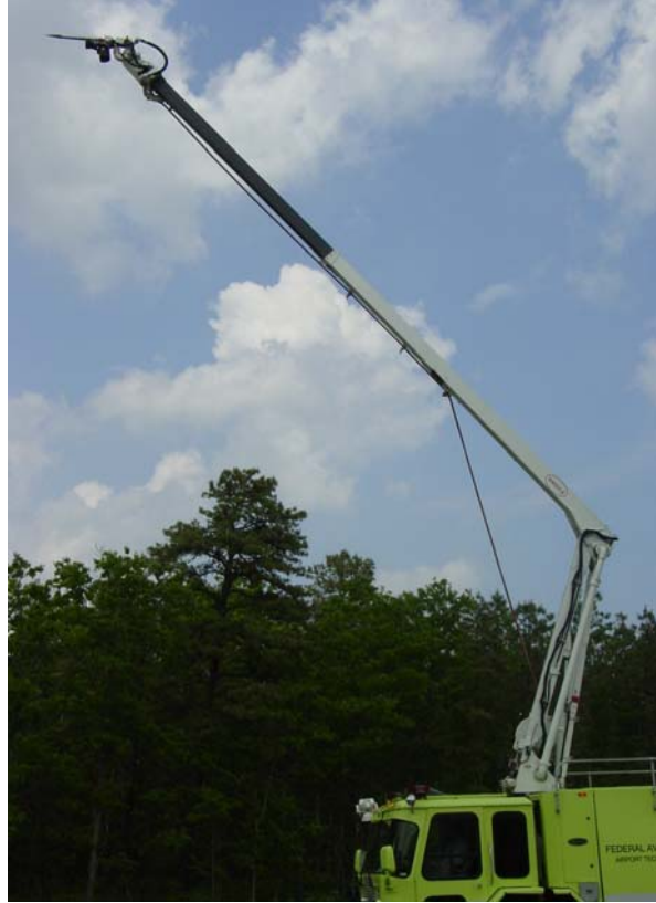
FIGURE 8. THE HPRV WITH HRET IN A FULLY ELEVATED, EXTENDED ATTACK MODE
