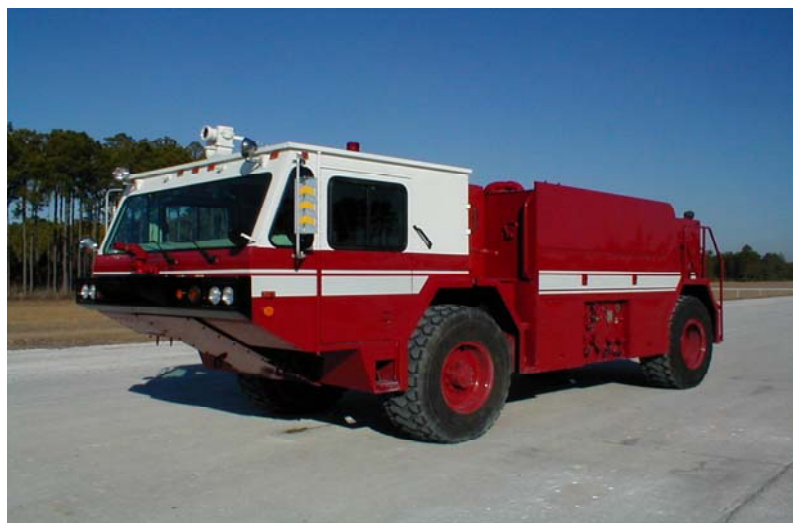
FIGURE 2. THE P-19 WITH ROOF-MOUNTED TURRET
