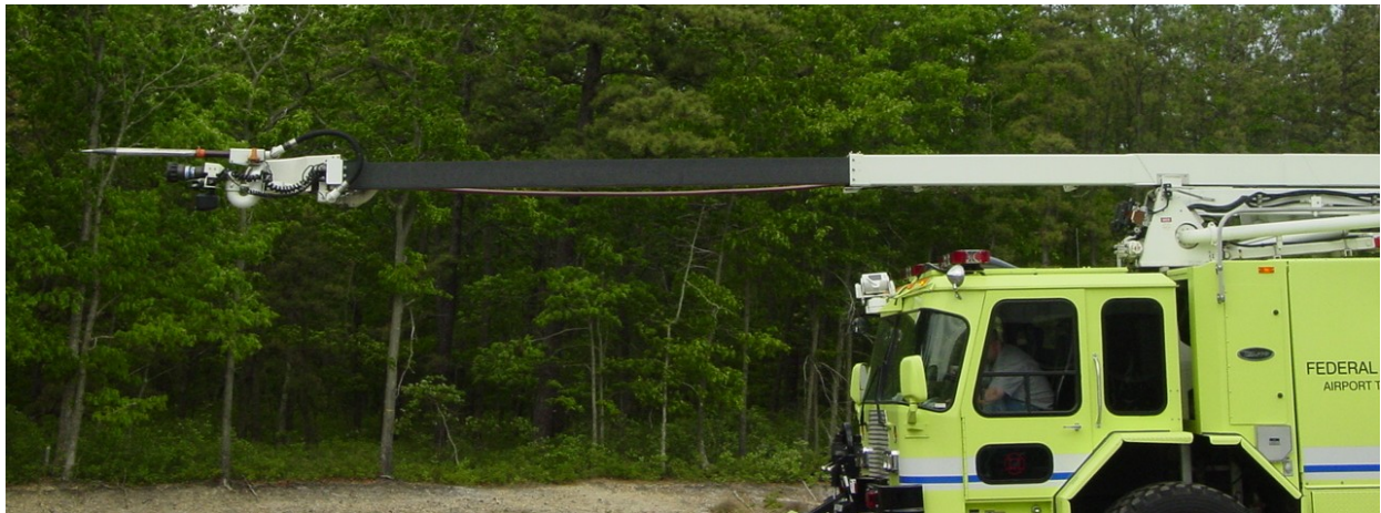
FIGURE 7. THE HPRV WITH HRET IN FULL FORWARD EXTENDED ATTACK MODE
