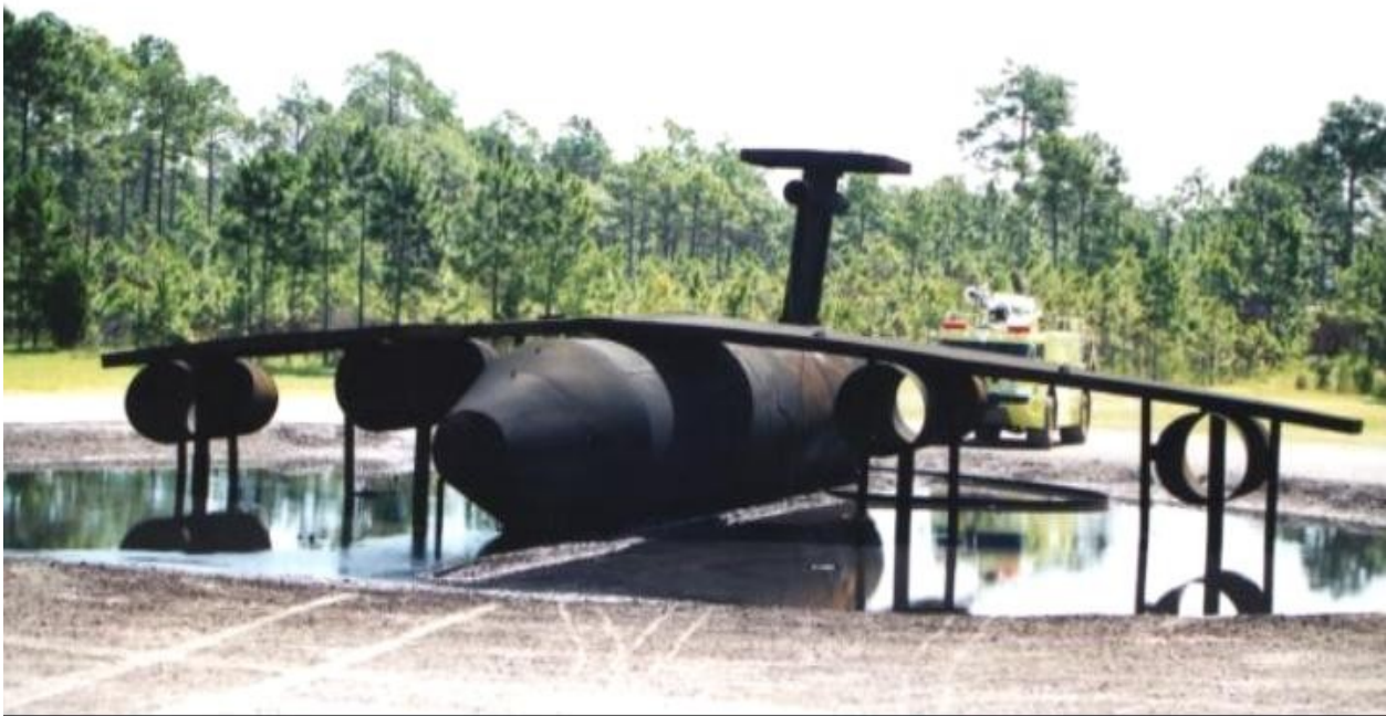
FIGURE 3. THE AFRL LARGE-SCALE, 100' DIAMETER TEST FACILITY WITH AIRCRAFT MOCKUP
