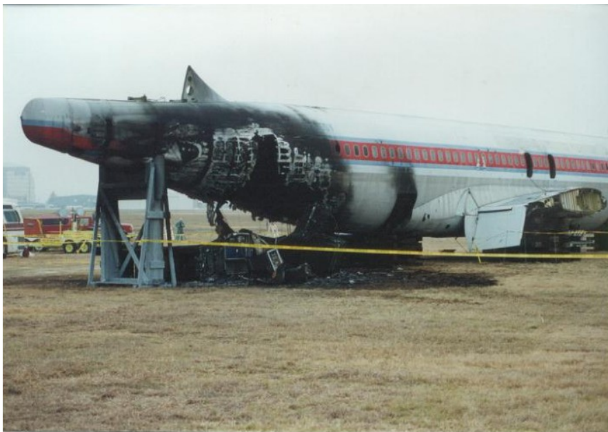
FIGURE 16. BURN-THROUGH AREA ON RIGHT SIDE OF AFT GALLEY AREA
