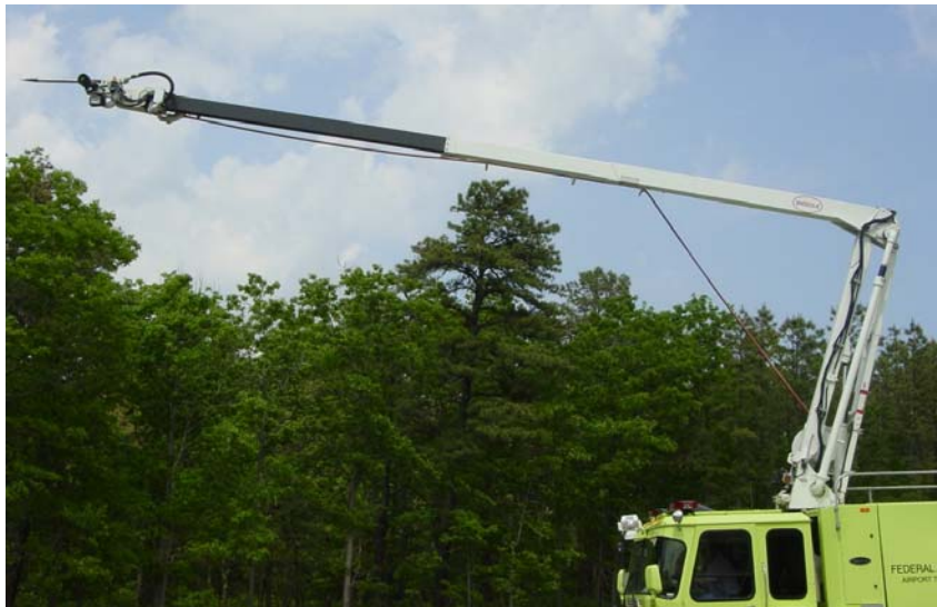
FIGURE 9. THE HRET IN A PENETRATING POSITION
