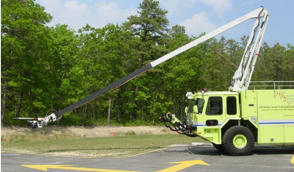
FIGURE 6. THE HPRV WITH HRET IN A DOWN-IN-FRONT ATTACK MODE
