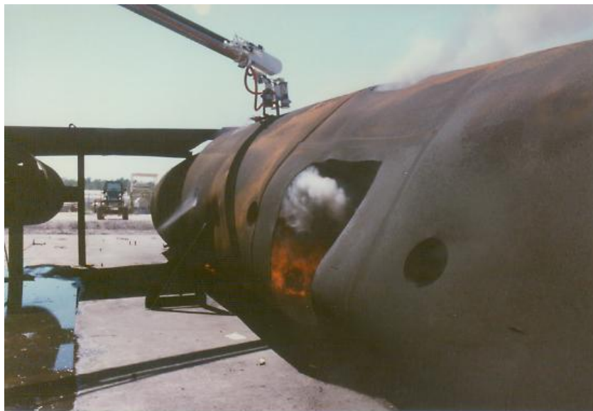
FIGURE 14. THE HPRV APPROACH WITH STANDARD SKIN-PENETRATING NOZZLE
