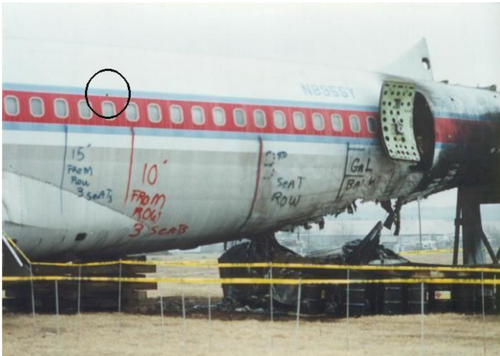
FIGURE 18. PENETRATION POINT ON LEFT SIDE OF FUSELAGE
