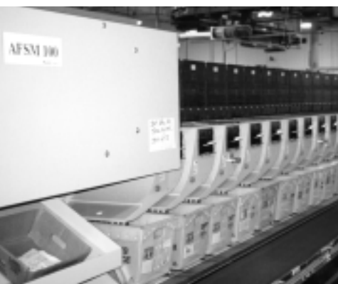
The OIG reviewed the deployment of the Automated Flat Sorting Machine 100, which automates processing of mail larger than a letter by incorporating on-site barcode technology.
