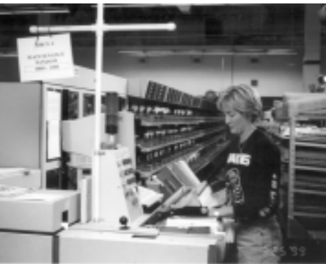
The OIG audits automation processes such as the Delivery Point Barcode sorter, which sorts mail in sequence of the letter carrier's route.
