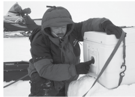
When researchers realized they had no way of knowing if the cameras were running within their insulated containers, a stethoscope solved the problem.
