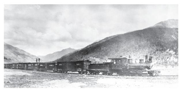
**Figure 9.** Silverton Northern Railroad and the Sunnyside mine's first "zinc train" (1915). Sunnyside began producing a zinc concentrate in 1915, which was shipped to a smelter out of the area. This special narrow gauge train was used to transport the powdered concentrate in 25-ton capacity boxcars, about half the size of standard gauge cars.
