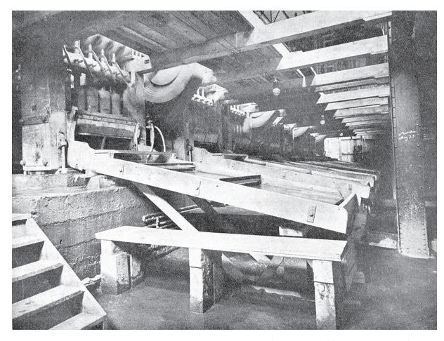
**Figure 12.** Stamps and mercury amalgamation plates, Old Hundred Mill (site # 238, fig. 2) (Silverton Miner, 1907). Inside the mills, heavy iron stamps pounded the ore to sand size, which washed over mercury-coated copper plates to catch the coarse gold and thence to concentrating tables.
