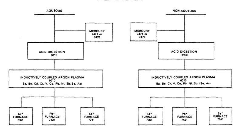
Figure 2: Schematic representation of the determination of metals in refinery samples.
