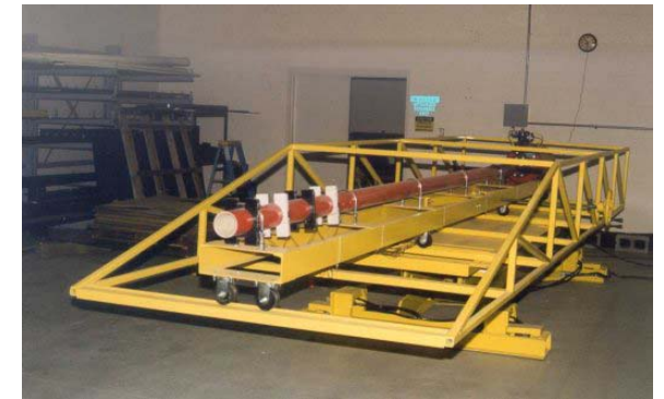
The Wind Science and Engineering Research Center at Texas Tech University tests various storm shelters and their components. One test uses this air cannon, which shoots 15-pound two-by-four wooden boards at shelter walls and doors to simulate flying debris. (Photo courtesy WISE)
