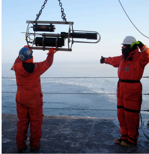
Figure 23. Philip Alatalo (L, WHOI) and Marine Science Officer LTJG Stephan Elliott (R, USCG) deploy the Video Plankton Recorder.
