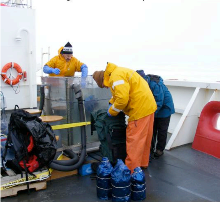
Figure 18. Ashjian/Campbell plankton wheel incubator, showing incubation bottles wrapped to simulate 15% in situ light level being placed on the plankton wheel. Bottles are slowly rotated for a 24 hour period while being immersed in flowing water at near surface seawater temperatures.
