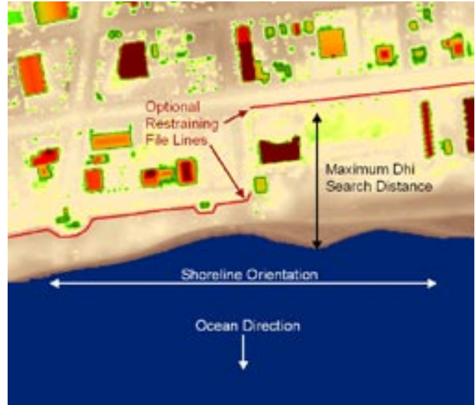
Figure 5. The required shoreline orientation, ocean direction, and maximum Dhi search distance parameters are illustrated in their required cardinal directions. Optional restraint lines, drawn here seaward of a seawall and a road, are also illustrated.
