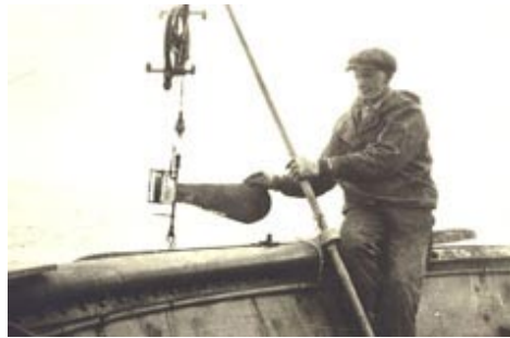
An oceanographer deploys a current meter in the 1920s while working in Alaska.
