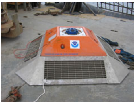
An Acoustic Doppler Current Profiler (ADCP) waiting to be deployed on the deck of a NOAA vessel. Click on the image for a larger view.
