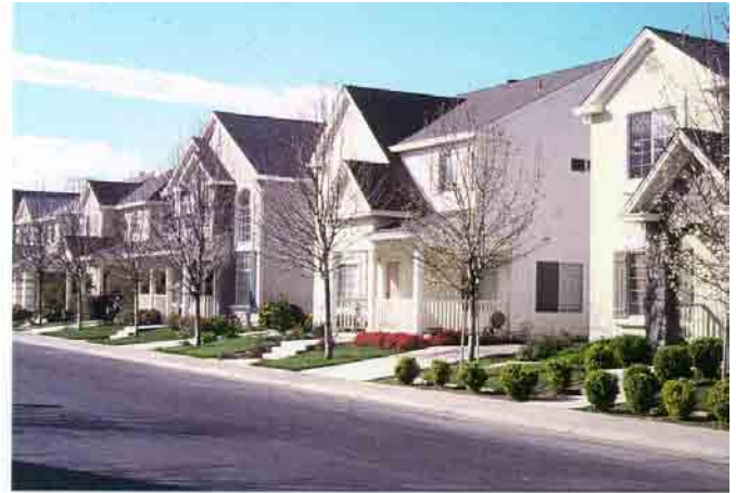
DGL 2.2.1: Front Yard Setbacks: Front yard setbacks may be as small as 7'-10' to the face of a front porch entry. The primary building front yard setback shall range from 10'-15' with single story facades being closer and two story facades having greater setbacks. A variety of setbacks is encouraged.
