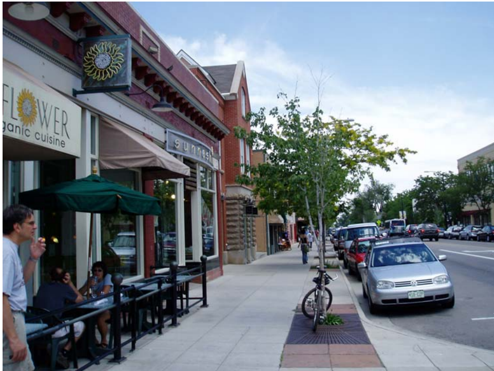
Figure 18: Examples of a “main street” design. Top photo is the Paseo del Pueblo Norte in Taos. Bottom photo is Pearl Street in Boulder. In both, note the on-street parking, the lack of driveways, and the vegetation that makes the street more attractive and comfortable for pedestrians.
