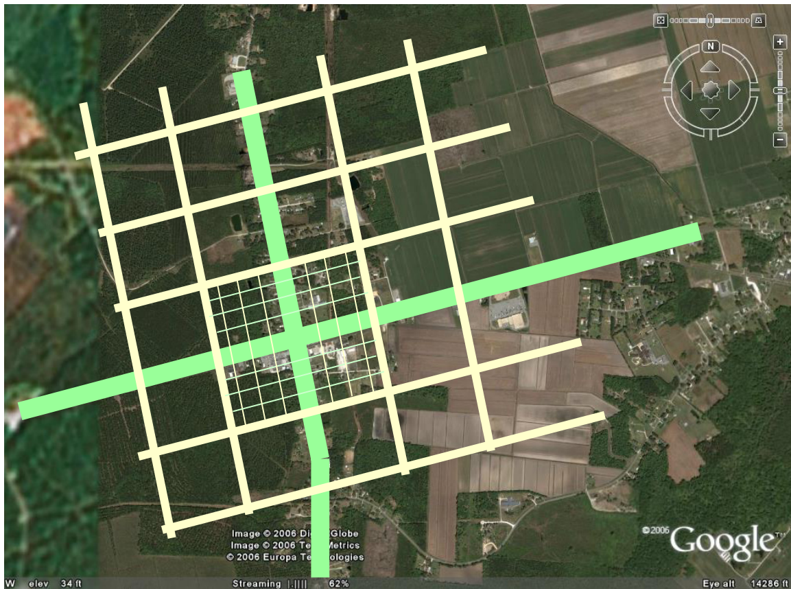
Figure 9. Depiction of a street network, rich in connections, imposed on an aerial photograph of the town of Grantsboro. The network demonstrates how alternative routes could reduce congestion on highway arterials. In this photo, the new streets are conceptual only, rather than specific places where the Team is recommending new streets be built. 14
