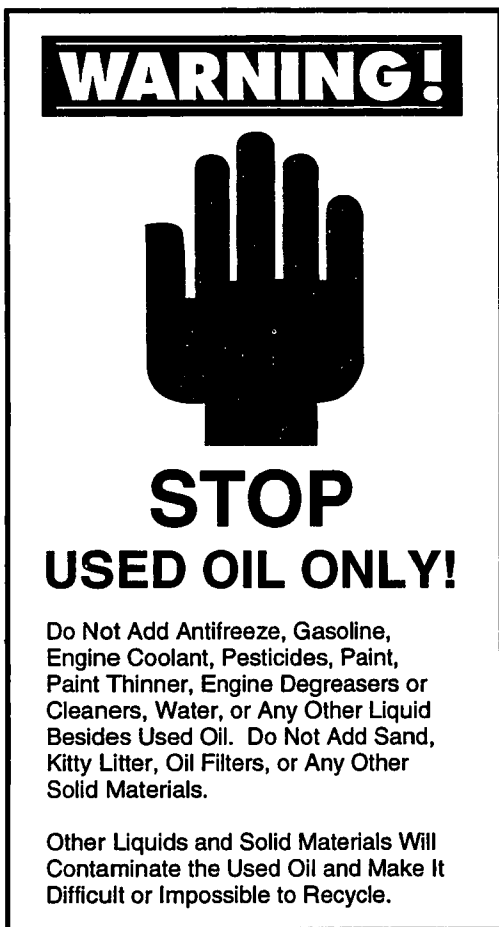
Figure 6-4. Label for used oil storage tanks and fill lines (source: adapted from Clean Burn, 1992).
