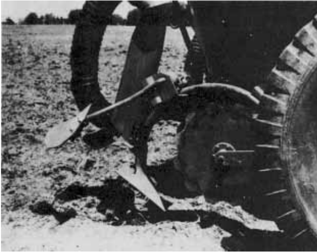
Figure 14-12a. Tank wagon with sweep shovel injectors (Cunningham and Northouse, 1981).
