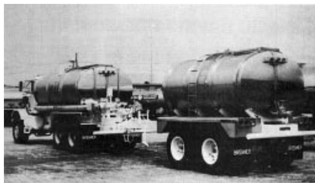
Figure 14-2b. A 3,300-gallon liquid sludge tank truck with 2,000-gallon pup trailer (courtesy of Brenner Tank Company).
