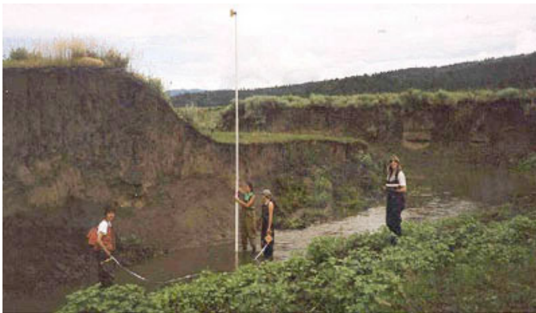
A field crew measures downcutting by a creek whose banks were trampled and destabilized by cattle. A lowered water table has reduced forage grasses in the adjacent pastures. Resident trout populations have also vanished.
