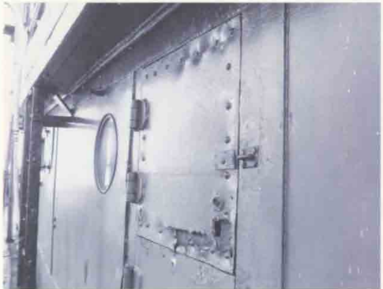
Fig. 21. Wastage typical of that seen in local areas of HERCULES' deckhouse.
