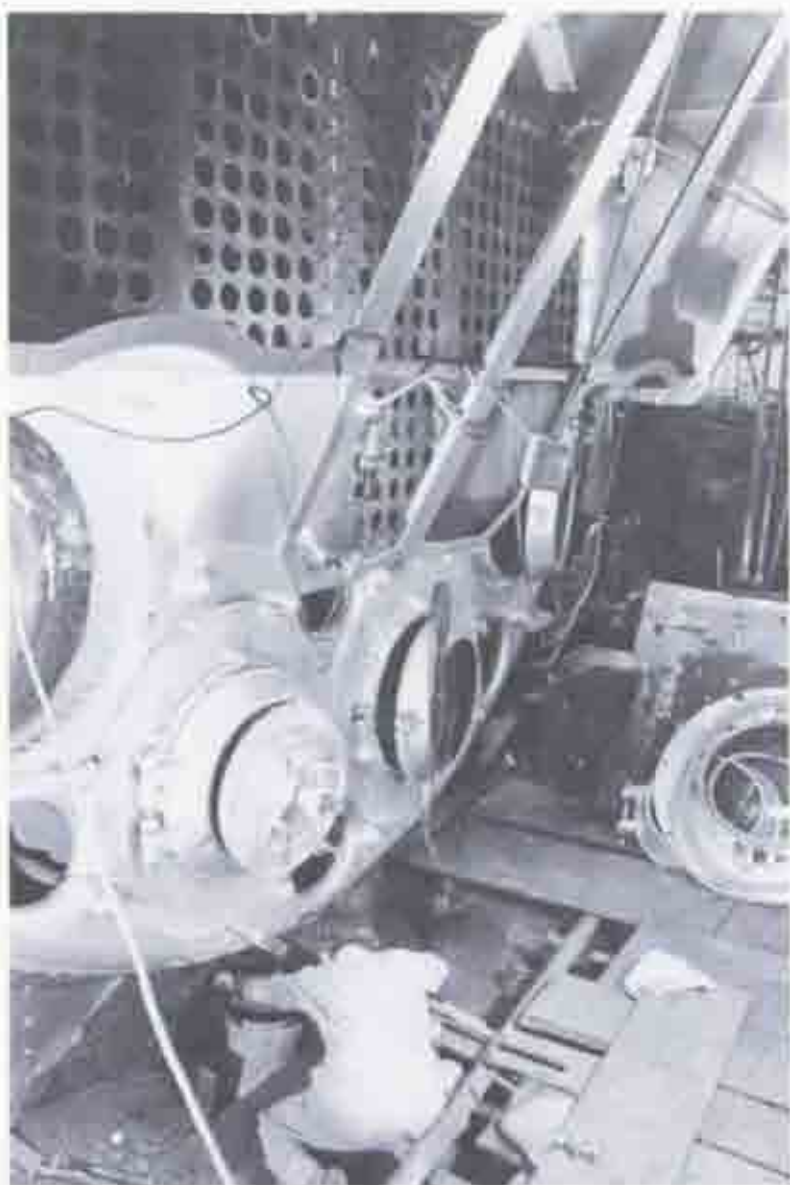
Fig. 22. View of the front end of HERCULES' boiler during restoration in the mid-1980s. Doors of the "front connection" have been removed for replacement of fire tubes.
