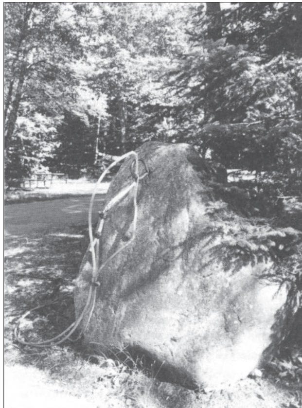
Figure 4.12. Similar boulder gates are used elsewhere in the national park system to control vehicular access, while avoiding introducing contemporary designed elements (ACAD, 1997).
