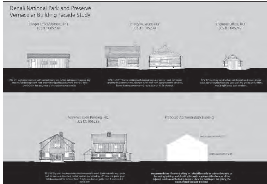
Figure 4.30. Buildings and Structures - Specify the mass and volume of the proposed new office facilities sympathetic to the design geometry of the existing historic buildings. Treatment Task 1.C - The proposed new building may avoid mimicking the materials of the historic buildings, and may employ energy-saving green technologies as care taken with building siting and mass and volume relationships will help the new building to fit appropriately into the context of the historic headquarters district (OCLP, 2006).
