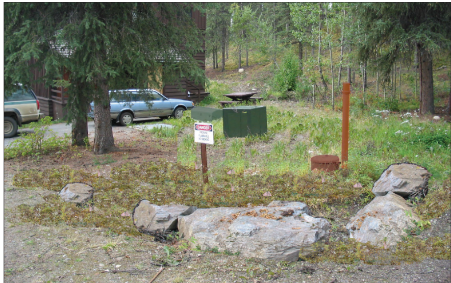
Figure 4.45. Small-Scale Features - Replace prominent safety bollards with appropriate rustic measures - Treatment Task 1.B - Replace non-historic steel bollards and otherwise visually prominent safety barriers with non-historic alternatives that are consistent with the historic character of the landscape. In this photo simulation, the visual prominence of both the barriers and the utility features are shown subordinated to the rustic character of the landscape. Refer to Figure 4.20 for specifications relating to size and installation (OCLP, 2007).
