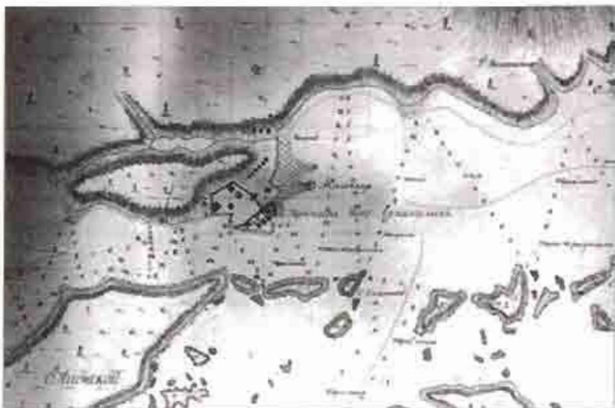
Map 5. Enlarged detail from "Karta zaliva Sitkhi..." [Chart of Sitka Sound, with all entrances to Novo-Arkhangel'sk port, latitude 57m2c48" N, longitude 135m13c51" W, newly corrected from a survey of the sloop Otkrytie in 1820 and 1821]. Depths are indicated in 7-foot sazhen. The inscription next to the circle in the center of the figure identifies it as the mill. The inscription below the mill states merely "Fortress Novo-Arkhangel'sk." The Indian River (R. Koloshenka) is at the upper right. (Limestone Press files, original in RGAVMF, Fond 1331, opis' 4, delo 181; previously published in Khlebnikov 1985, facing p. 57.)
