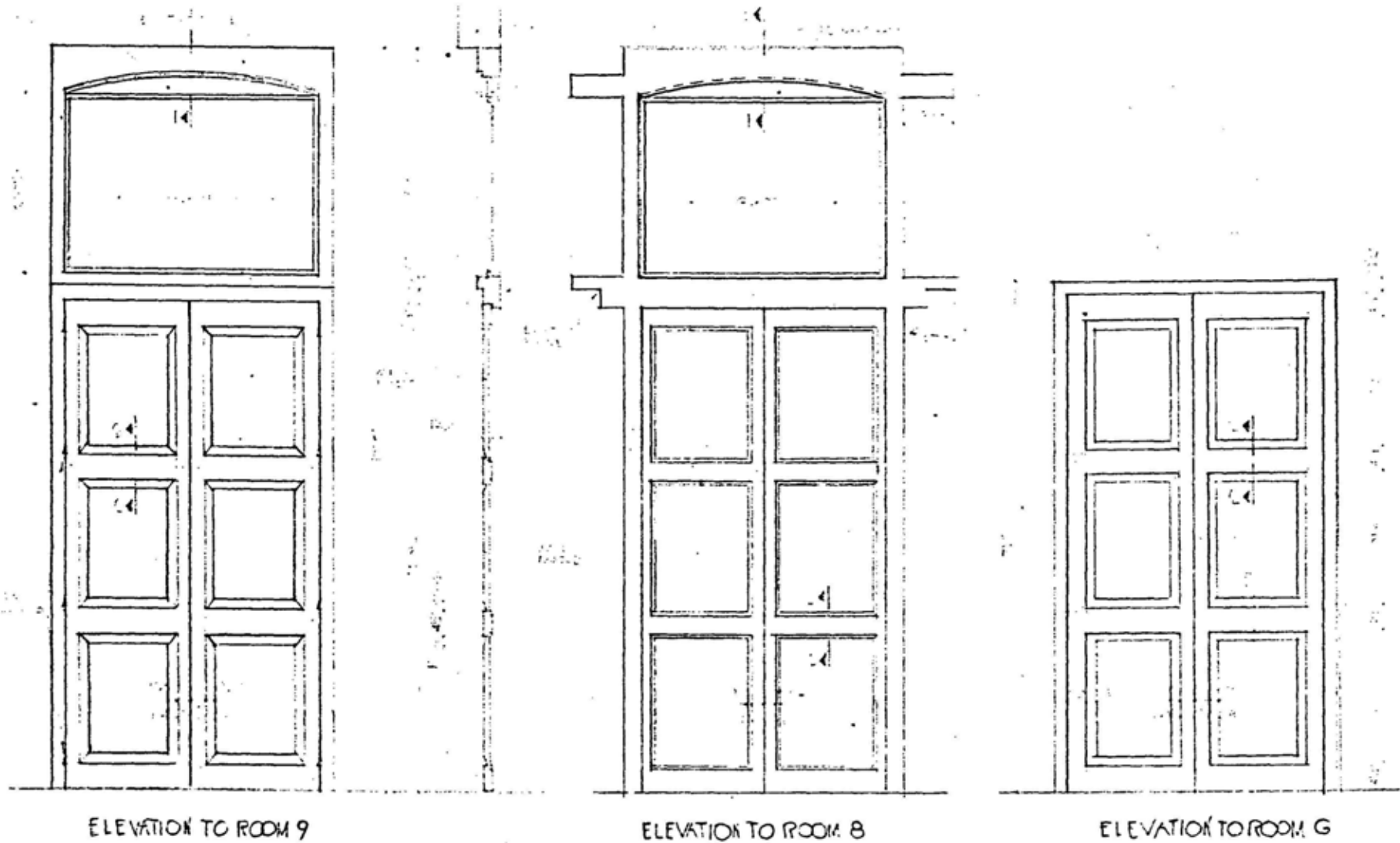
Figure 17b. Door type "D", San Cristóbal. (Dept. of Interior, Division of Design and Construction. Drawing no. NHS: SJ/3062, 1962.)
