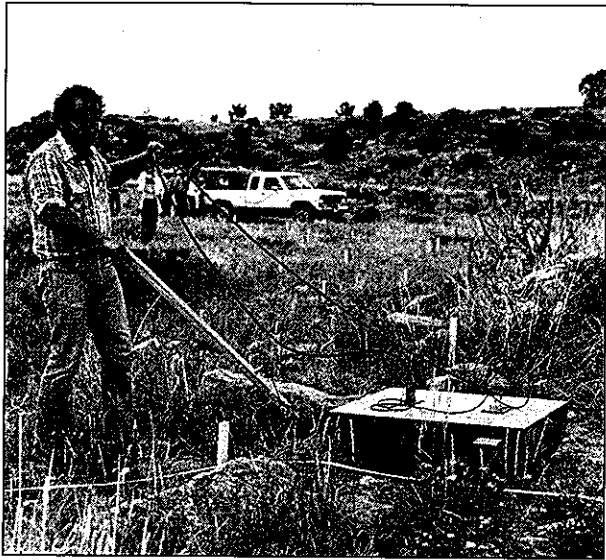
Figure 5. A ground penetrating radar being pulled across the ground. Lockwood Stage Stop, Pinon Canon Maneuver Site, Colorado. (NPS, 1991)
