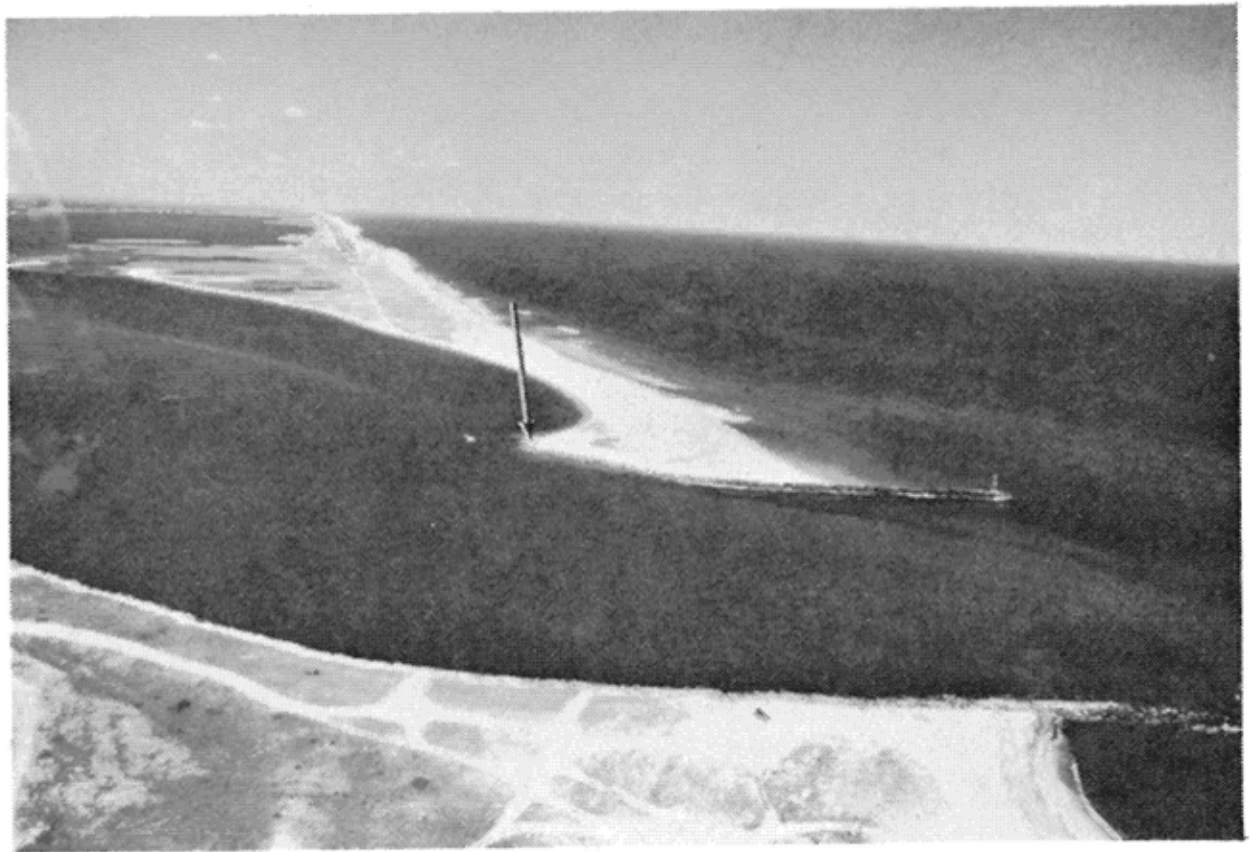
Figure 8. Moriches Inlet, Long Island, New York, looking east June 1978. Note relative position of oceanfront shorelines in this figure and Figure 9. The base of the eastern jetty is marked with an arrow in each figure.
