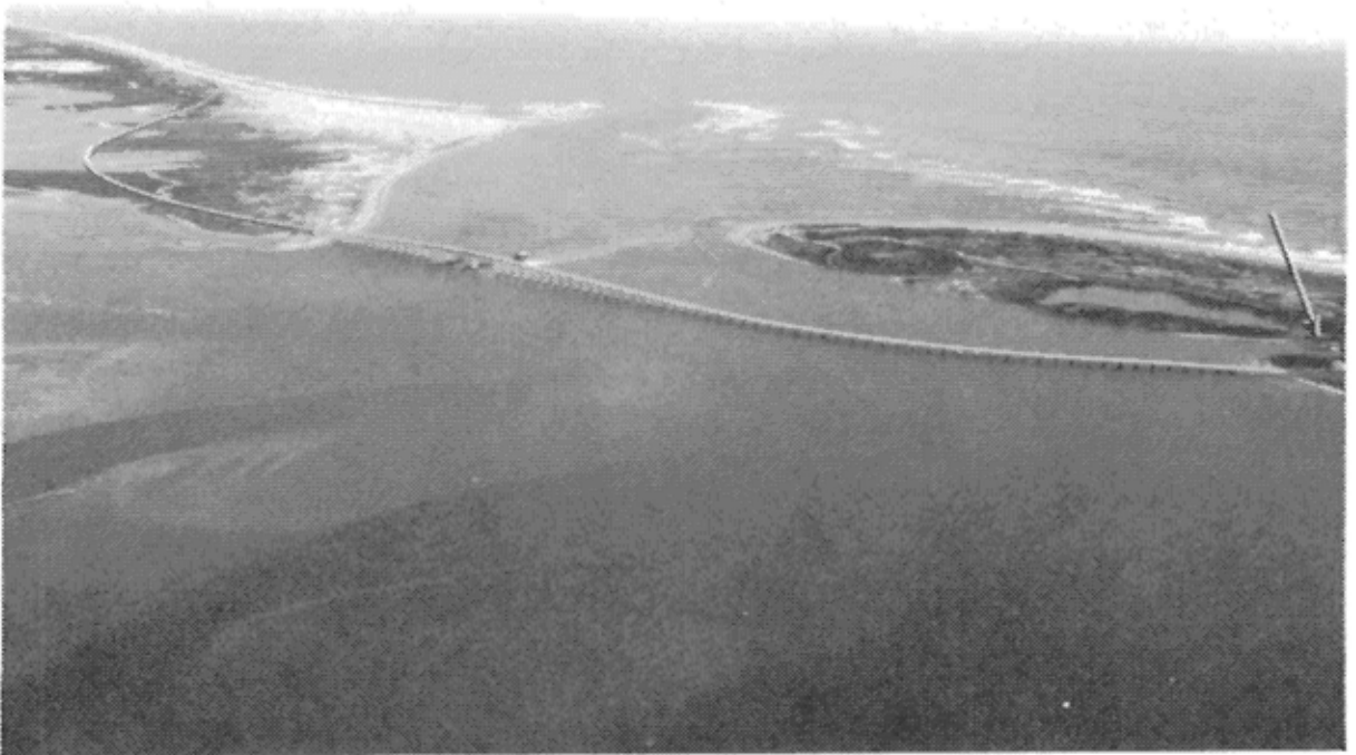
Figure 6. Oregon Inlet, Outer Banks of North Carolina, December 1979, (a) looking south and (b) looking north. Arrow marks Coast Guard station threatened by erosion as inlet migrates southward.
