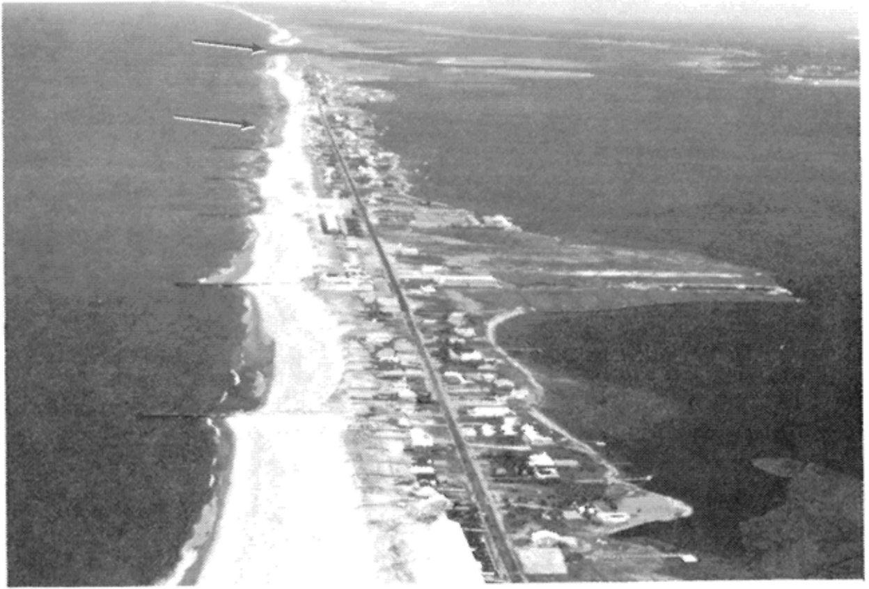
Figure 7. Westhampton Beach, Long Island, New York, looking west-southwest in June 1978. Note erosional shadow downdrift of last groin (near arrow), and new inlet breach at Moriches Inlet (far arrow). See also Figures 8 and 9.
