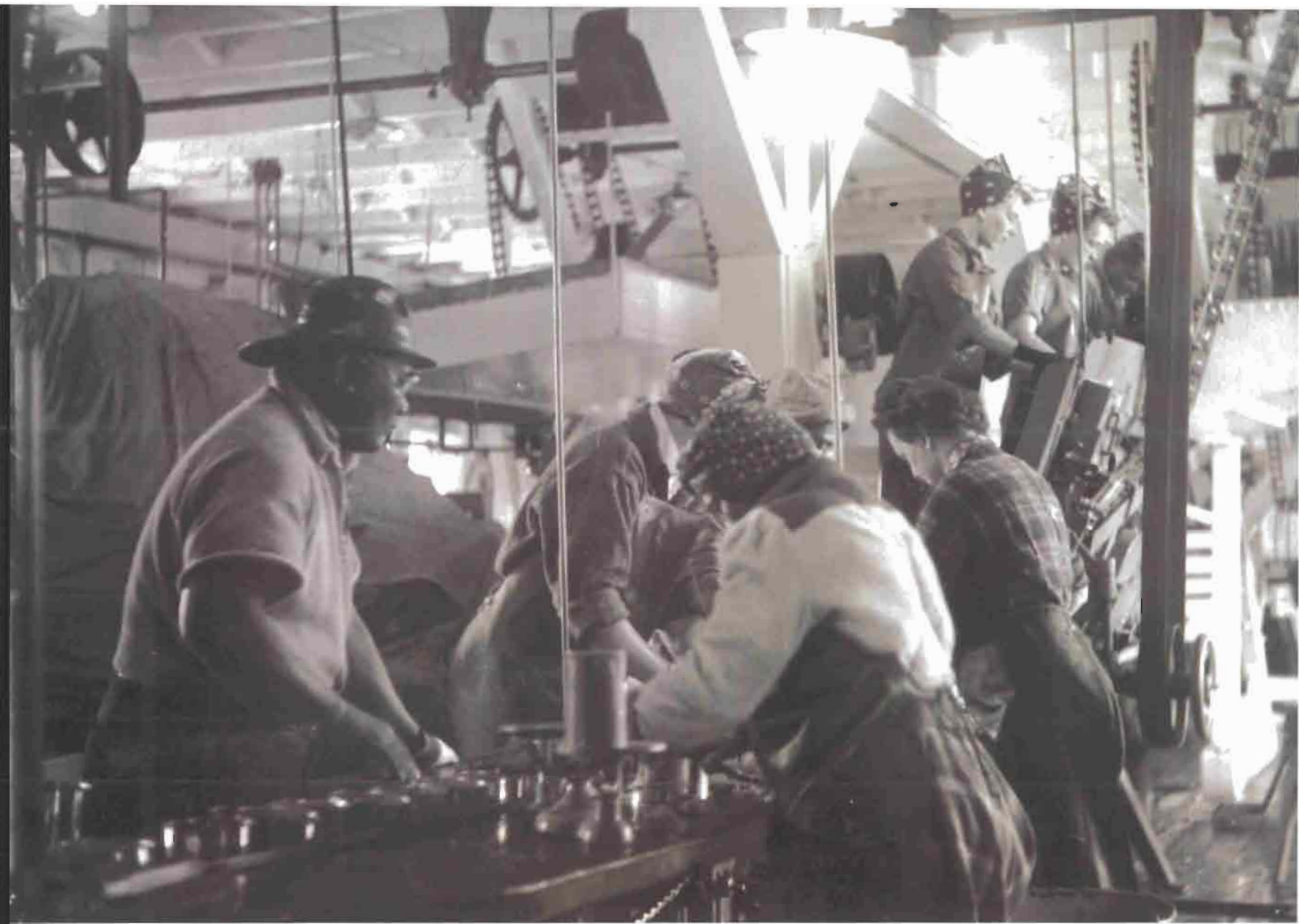
"In the foreground is the 'patch table' where small pieces of salmon are inserted in cans imperfectly filled by machinery," The Alaska Sportsman, August 1953.
