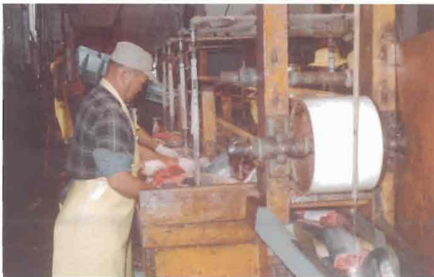
"Sliming table," Each fish is hand-washed and blood from the backbone is removed after the fish pass through the "Iron Chink" machine that decapitates heads and removes fish guts. Courtesy of Dorothy Fribrock, private collection.
