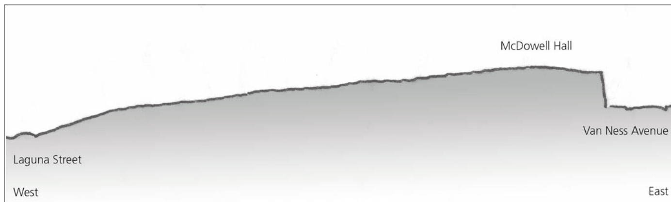
Figure 3.1.11: Topographic diagram. This drawing shows the shape of the land, in cross-section along the approximate east/west alignment of MacArthur Avenue. 1"=300'. Vertically exaggerated 3:1. OCLP.
