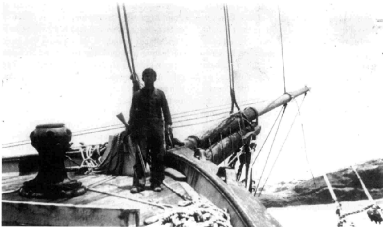
Figure 3.13. Unidentified man on Comet's forecastle deck. Note the capstan which is still mounted in the same location today. Also, note the rock ledge in the background which can be compared to Figure 3.14. Photo courtesy of Santa Barbara Museum of Natural History.
