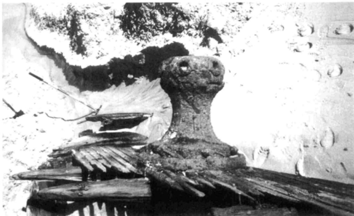
Figure 4.103. Comet's capstan, mounted in the center of the forecandle deck. NPS photo by Don Morris.
