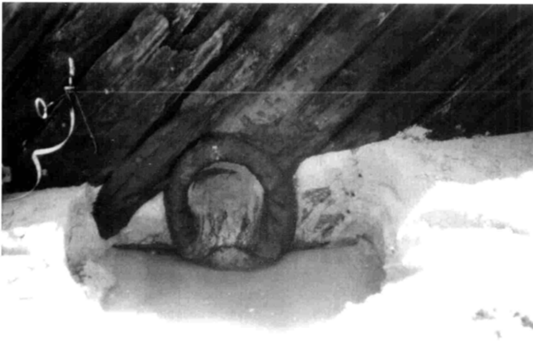
Figure 4.102. Comet's port-side hawse pipe. NPS photo by Don Morris.
