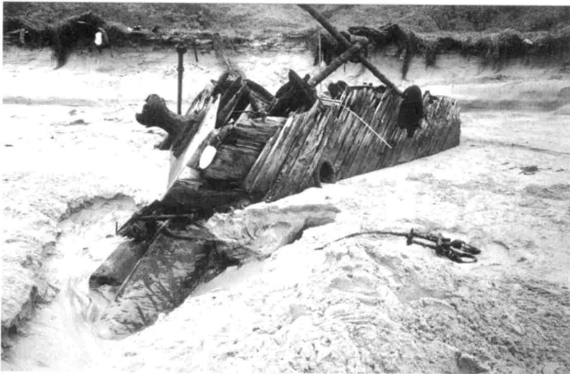
Figure 4.75. Comet's bow. The hawse timbers are in the center with the white float on them. The hawse pipe is visible at the sand-line, to the right of the hawse timbers. In the right foreground is an unattached rigging element. NPS photo by Matt Russell.
