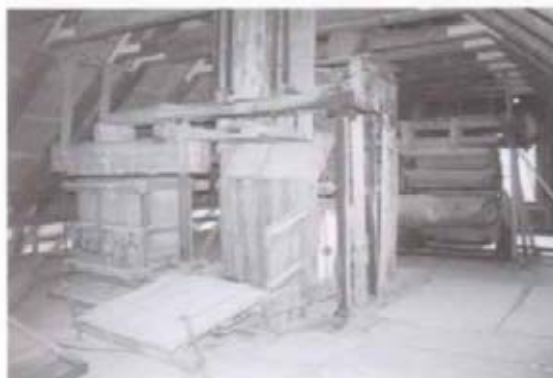
Figure 44 View east of dual-box hydraulic press at second floor, with gin stand visible in background. (NPS-SERO-CRS, 2001)
