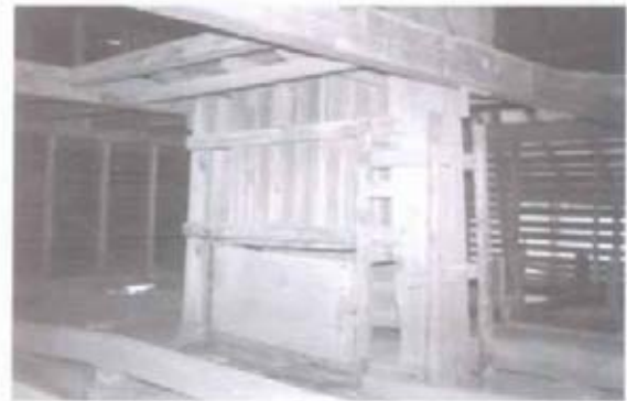
Figure 46 View of cotton press at ground level, showing door where finished bale was removed. (NPS-SERO-CRS, 2001)
