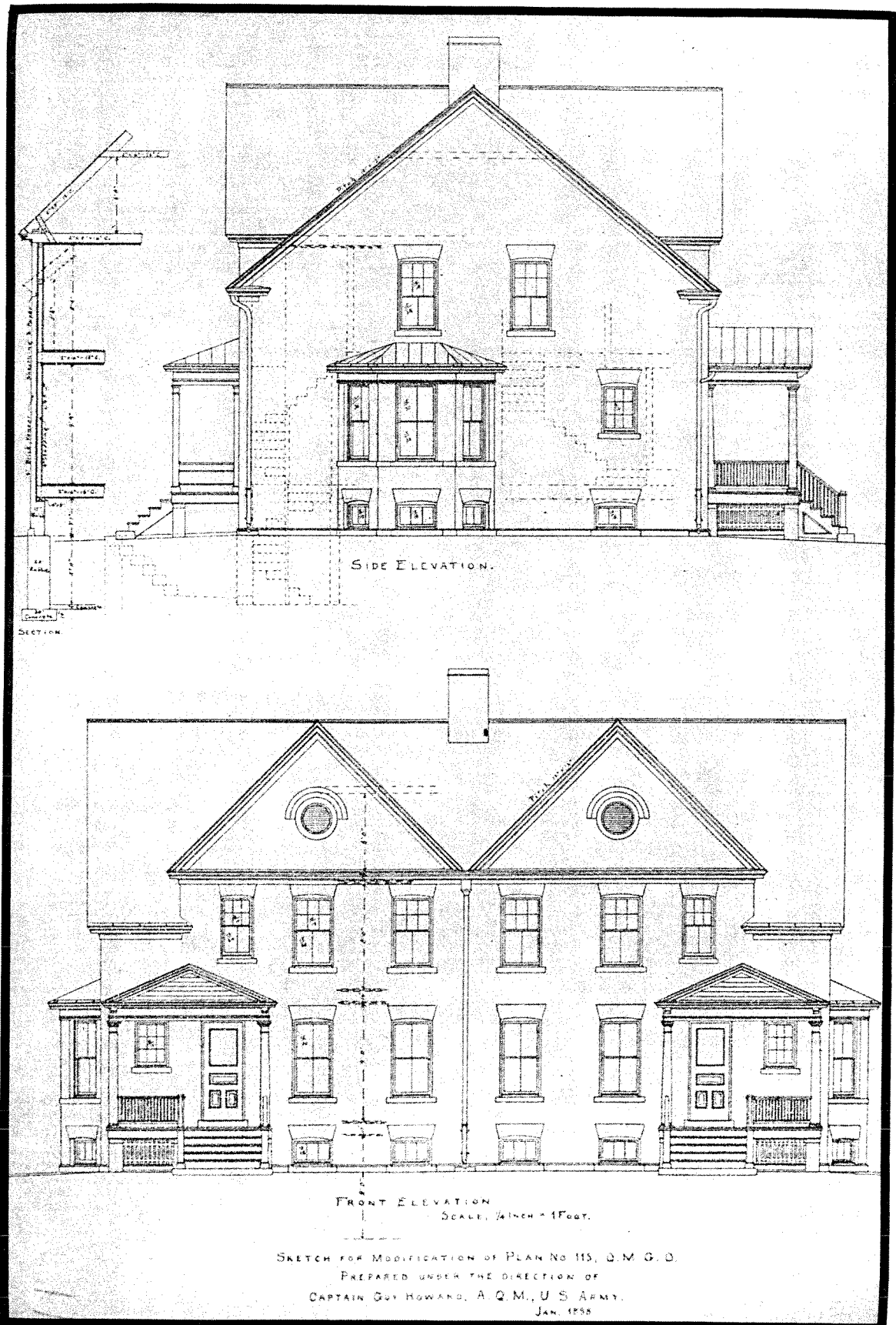
Figure I-6. 1897 Quartermaster Department standardized plan for double set of brick officers' quarters. Known locations: Ft. Omaha, Nebraska; Ft. Leavenworth, Kansas; Jefferson Barracks, Missouri; Ft. Porter, New York; Ft. Brady, Michigan; and, Ft. Ethan Allen, Vermont. (From Grashof, Standardized Plans 1866 - 1940 , Vol. 3, 1986; original drawing source: National Archives, Cartographic and Architectural Branch, RG 77, P.I. NM-19, E. 411-#115)
