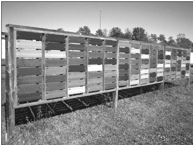
Figure 26—Extruded composite boards manufactured with pine wood flour, juniper wood flour, and saltcedar wood flour on a test rack for natural weathering in Madison, Wisconsin.
