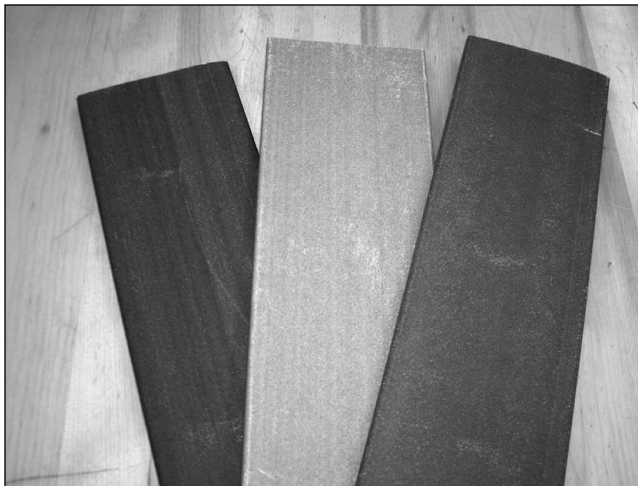
Figure 20—Extruded boards of HDPE containing 50% saltcedar (left), pine (center), or juniper (right) and lubricant and no coupling agent or UV package. See Table 2 for details on formulations.
