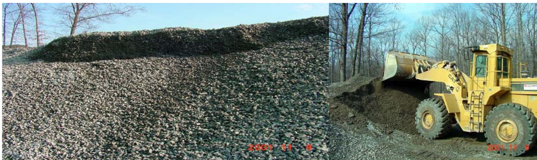
3-16 Aggregate Separation In A Pile Is Normal
