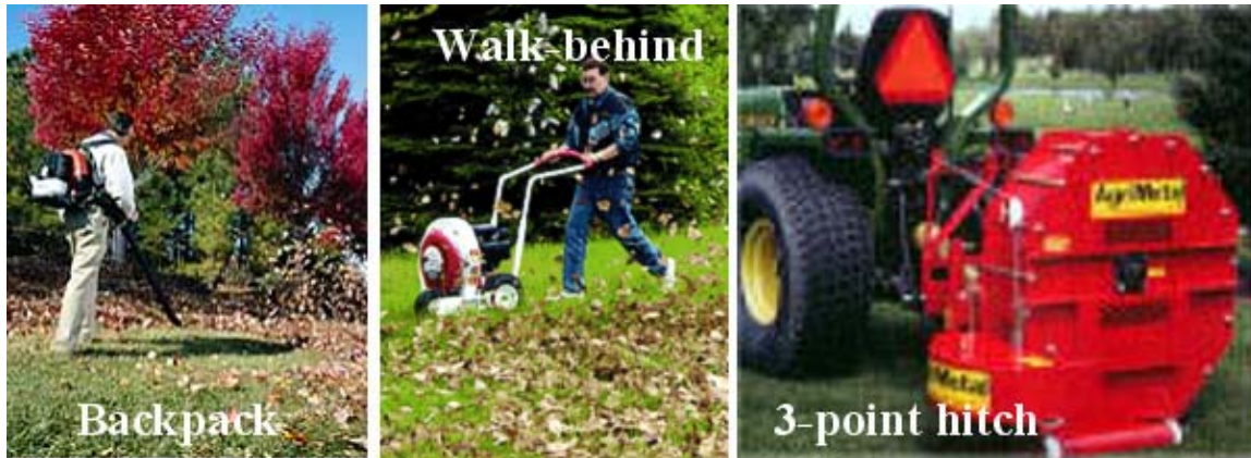
6-14 Leaf Blowers to Clean Ditches and the Roadway
