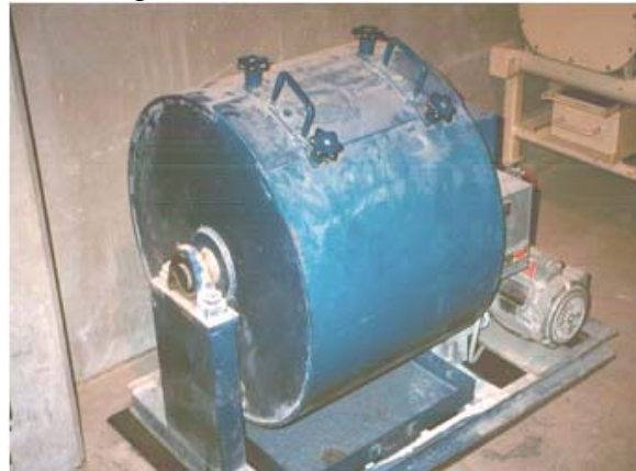
2 - 11 Los Angeles Abrasion Test Drum.
