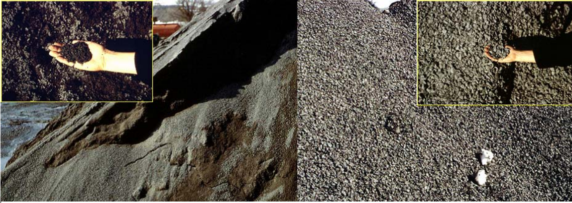
3-12 A good road surface aggregate will be well graded from fine to coarse.
