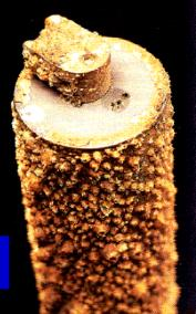
Turbidity sensor after deployment for 30 days
