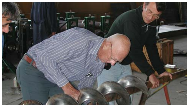
Volunteer Gordon Schmidt, left, from Henderson, Nebraska, and client Todor Toporov, work on a grain storage bin auger in Toporov's shop in Silistra, Bulgaria.
