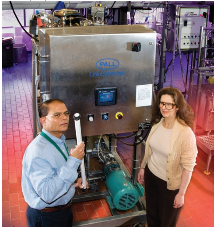
ERRC chemical engineers Sudarsan Mukhopadhyay (left) and Peggy Tomasula examine a ceramic membrane module for use in microfiltration of liquid egg whites to eliminate potential pathogens such as Salmonella enteritidis .
